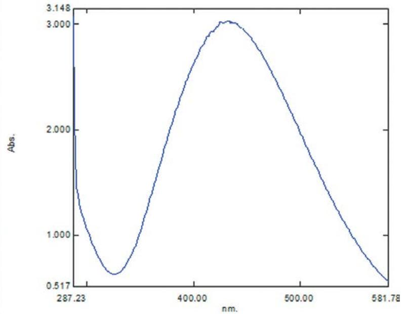
**Figure 2.** UV-Vis spectra analysis of silver nanoparticles.
