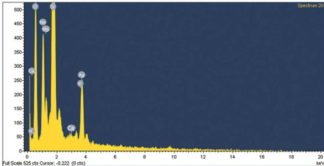
**Figure 4.** Energy dispersive X-ray Analysis of silver nanoparticles.
