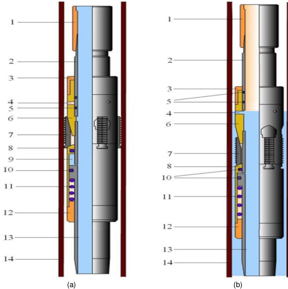
**Figure 1.** Schematic of a hydraulic anchor. at (a) Anchoring status and (b) Releasing status, 1- Upper joint; 2-Oil drainage nipple; 3-Upper protection cap; 4-Drain hole; 5-Seal ring; 6-Taper; 7-Slips; 8-Piston; 9-Hydraulic cavity; 10-Seal ring; 11-Spring; 12-Lower protection cap; 13-Centre tube; 14-Casing.
