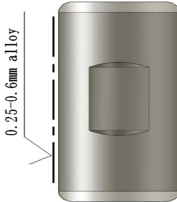
**Figure 2.** Coupling with circular arc and coating with alloy.
