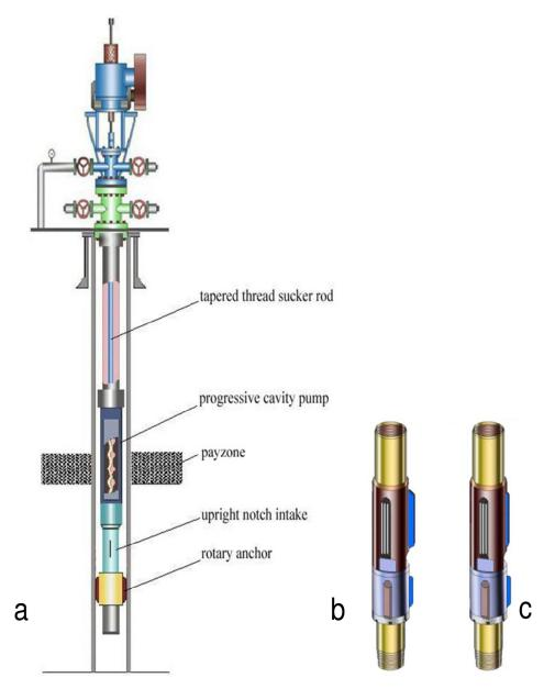
**Figure 4.** (a) Schematic of the modified PCP system together with pump intake configuration: (b) Rotary anchor in operational state, and (c) Rotary anchor in idle state.
