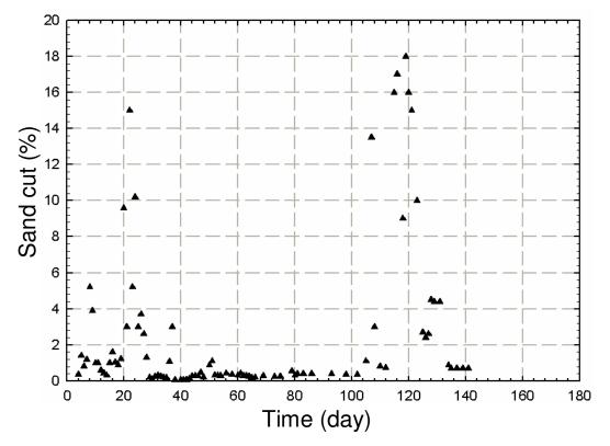
Figure 6. Produced sand cut as a function of time for Well X7-14.
