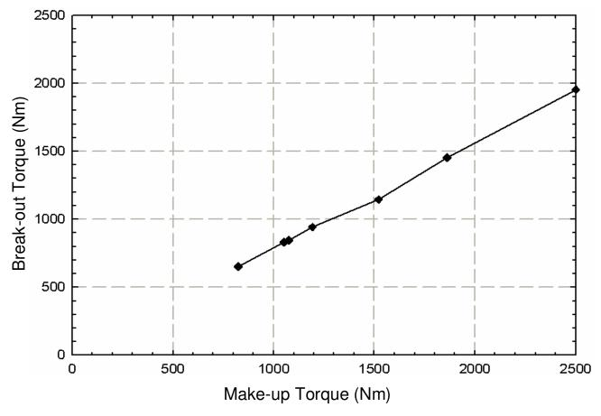
Figure 3. Measured make-up and break-out torques.
