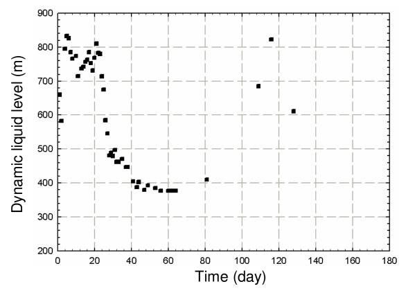
Figure 7. Producing fluid level as a function of time for well X7-14.
