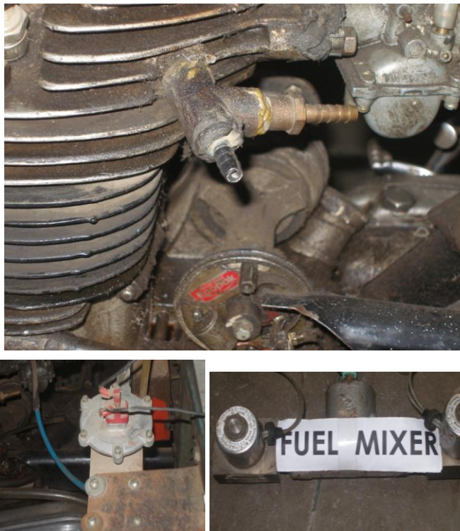
Figure 3. Fuel mixer with locally designed gas supply control and view of gas injection system at manifold.
