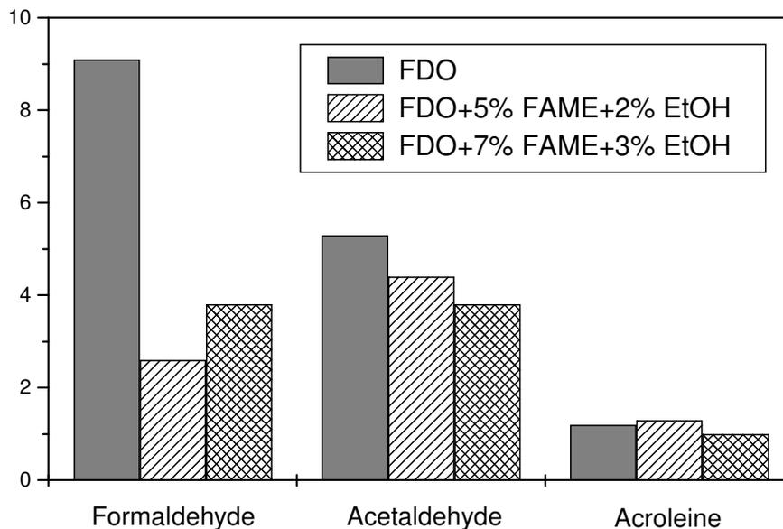
**Figure 1.** Concentration of formaldehyde, acetaldehyde and acroleine in  $\mu\text{g/l}$  in exhaust gases at maximum engine revolutions and at half load of the engine measured on MD UR IV engine. Water content in EtOH 0.7% w/w.
