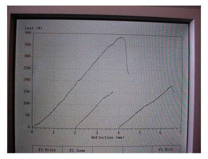
Figure 4. A typical load-deformation curve of palm kernel under horizontal compressive loading.
