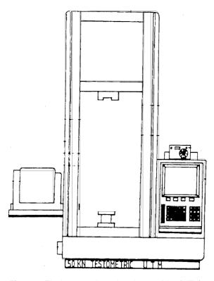
Figure 3. The instron universal testing machine (UTM).
