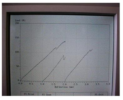
**Figure 5.** A typical load-deformation curve of palm kernel under vertical compressive loading.
