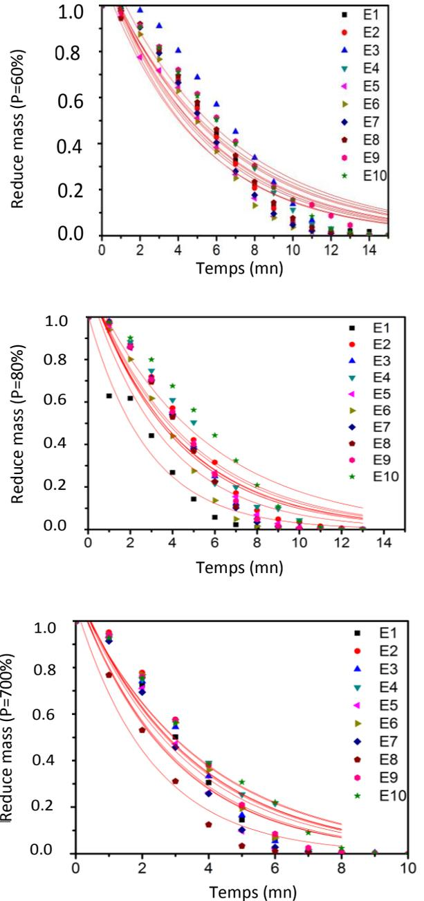
**Figure 5.** Microwave drying curves of fresh safou pulp based on diffusional model.
