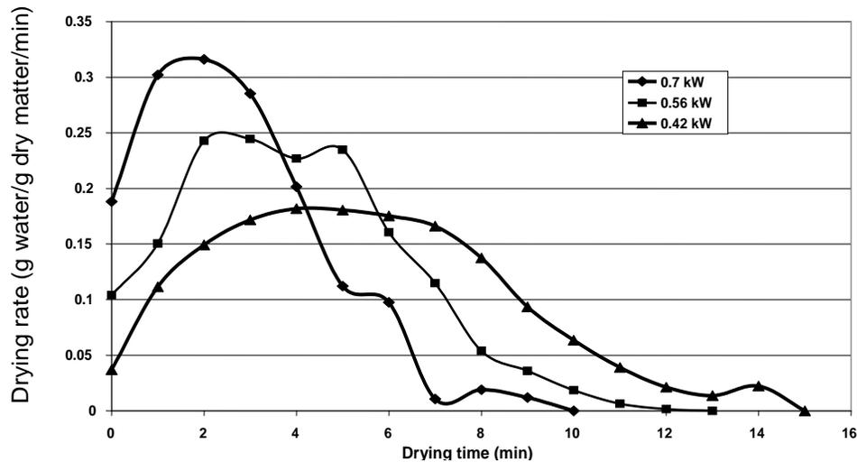
**Figure 2.** The relations of drying rate and time in drying of fresh samples.
