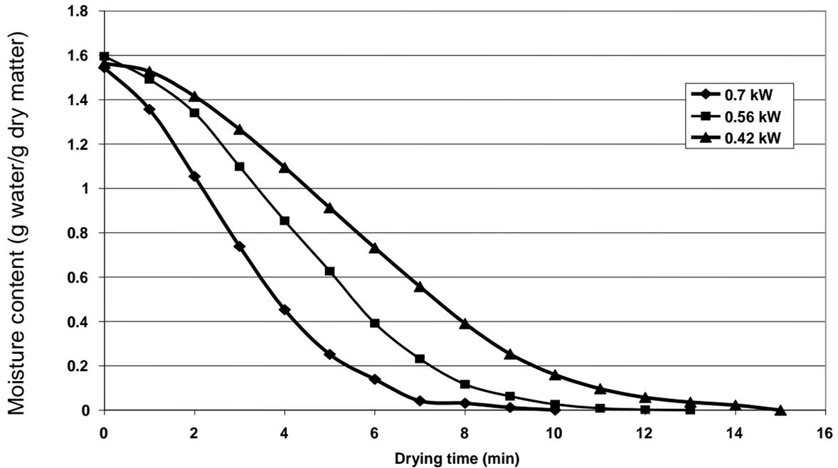
Figure 1. Drying curves of fresh safou pulp at different microwave powers.
