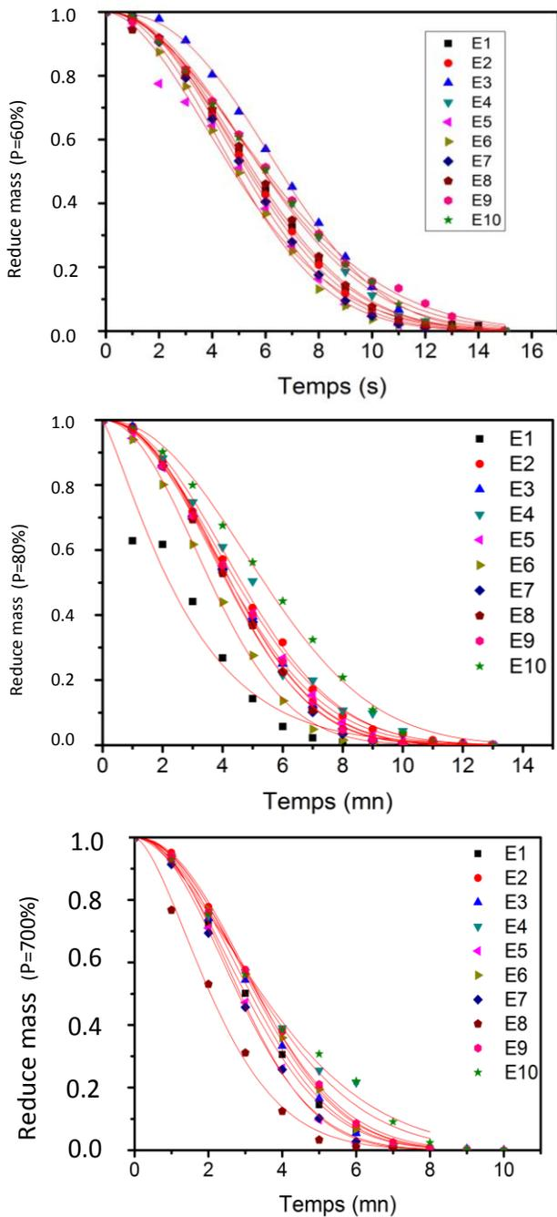
**Figure 4.** Microwave drying curves of fresh safou pulp based on Avrami model.
