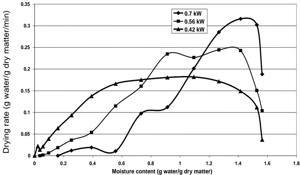
Figure 3. Drying rate of safou pulp at different microwave powers.
