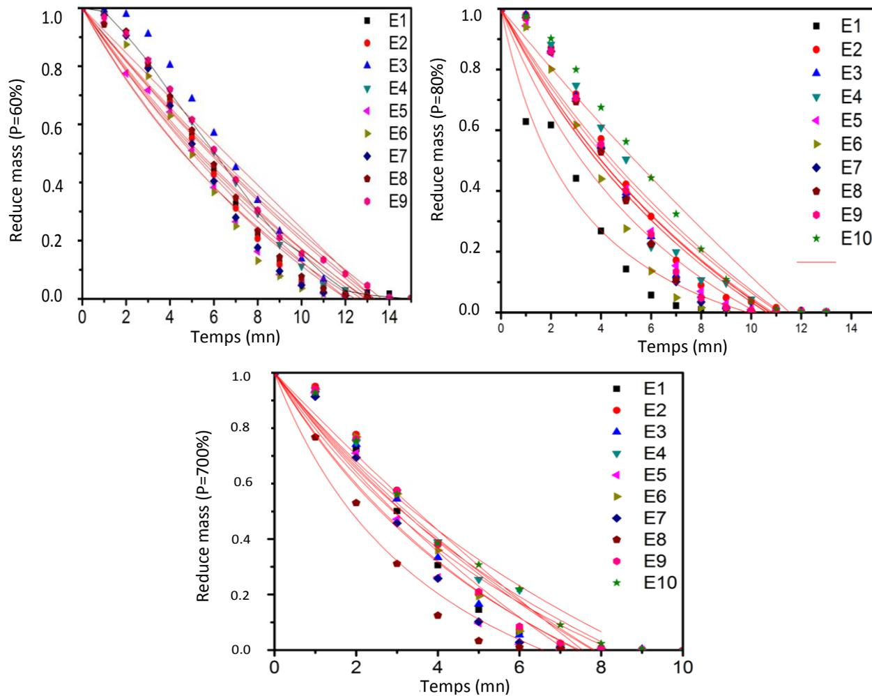
Figure 6. Microwave drying curves of fresh safou pulp based on Peleg model.
