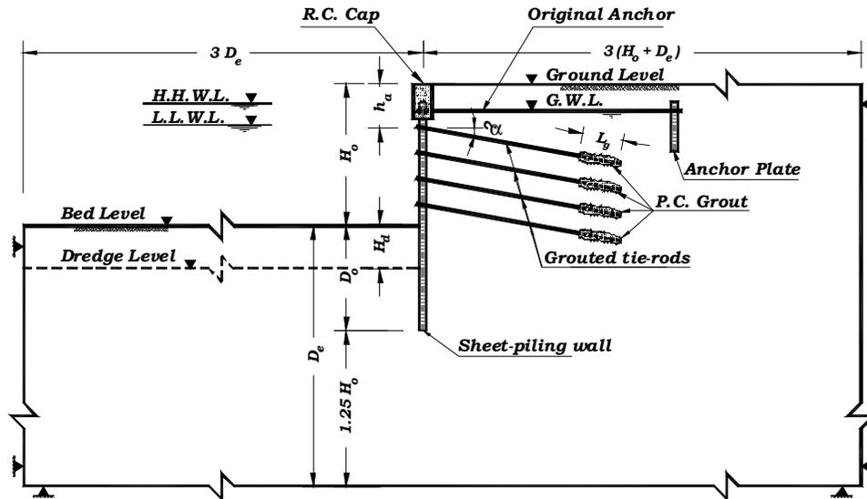
Figure 1. Geometry of Multi-Anchored-Sheet Pile System.
