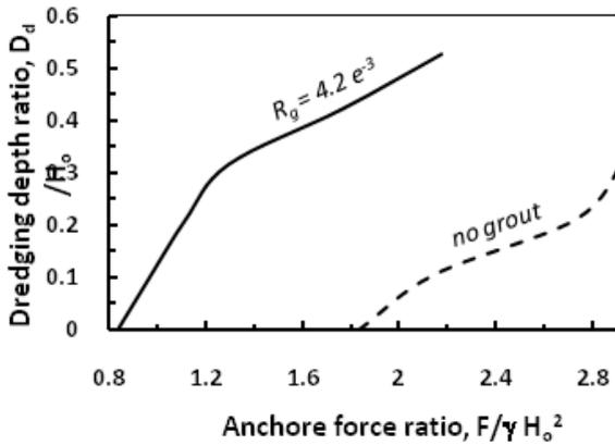
**Figure 12.** Maximum anchor force ratio,  $R_F$  versus dredging depth ratio,  $R_d$ .
