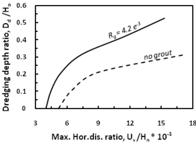
**Figure 13.** Maximum horizontal displacement ratio,  $R_{ux}$  versus dredging depth ratio,  $R_d$ .
