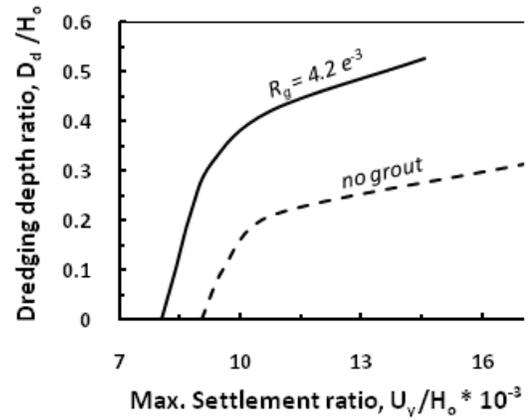
**Figure 14.** Maximum settlement ratio,  $R_{uy}$  versus dredging depth ratio,  $R_d$ .
