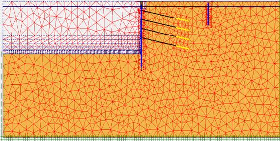
**Figure 2.** Finite Element Model as Generated by PLAXIS.
