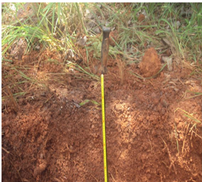
Figure 2. Gravelly soil profile observed in Bagoé watershed, Sikasso region (Photo I: Kassogué).
