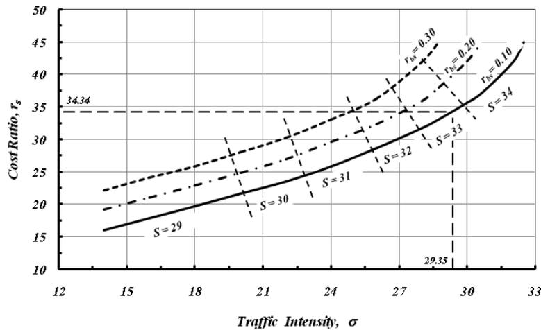
Figure 8. Determination of Optimum Number of Berths,  $\sigma$  due to different cost ratio,  $r_{bs}$ , Alexandria Port, Case Study.
