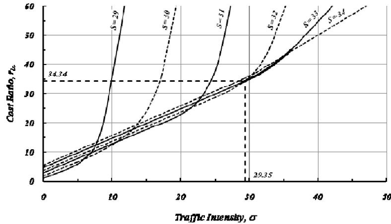
Figure 7. Determination of optimum number of berths,  $\sigma$ , Alexandria port, case study.
