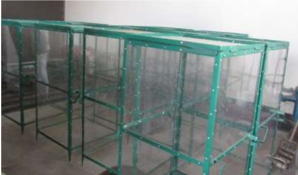
Figure 1. Static closed chamber for trapping methane in rice soil.
