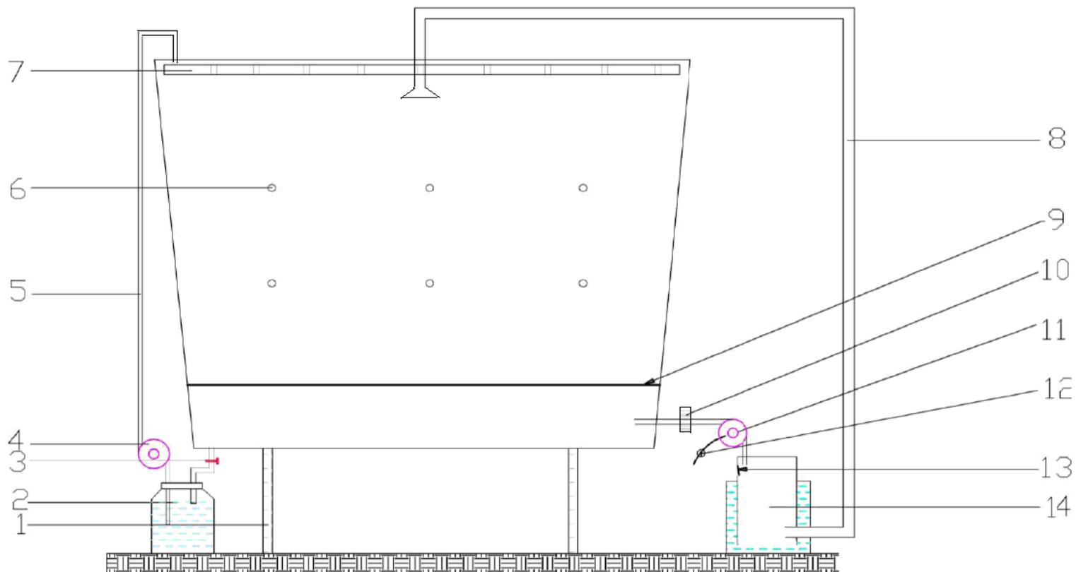
**Figure 1.** Schematic diagram of aerobic composting device; 1.support, 2.bucket, 3.valve, 4.pump, 5.water pipe, 6.hole for thermometer, 7.water spray, 8.wind pipe, 9.gas separation plate, 10. gas flowmeter, 11.fan, 12. time relay, 13.baffle,14. gas reservoir.
