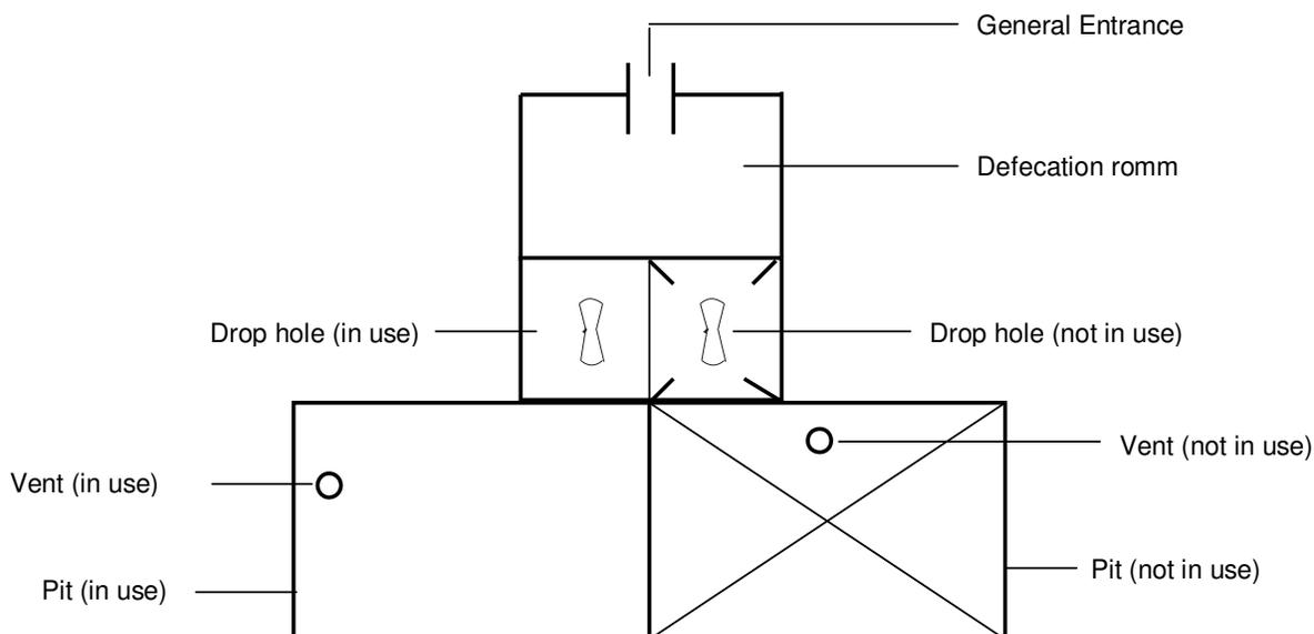
**Figure 1.** Plan view of domestic alternating pit (VIP latrine).
