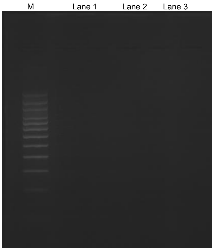
Figure 3. Agarose gel electrophoregram of PCR products of DNase treated RNA extracted from A. niger using TRIZOL with RNaseOUT. M is the molecular weight marker lane, Lanes 1, 2 and 3 were loaded with the PCR products but no bands appeared.
