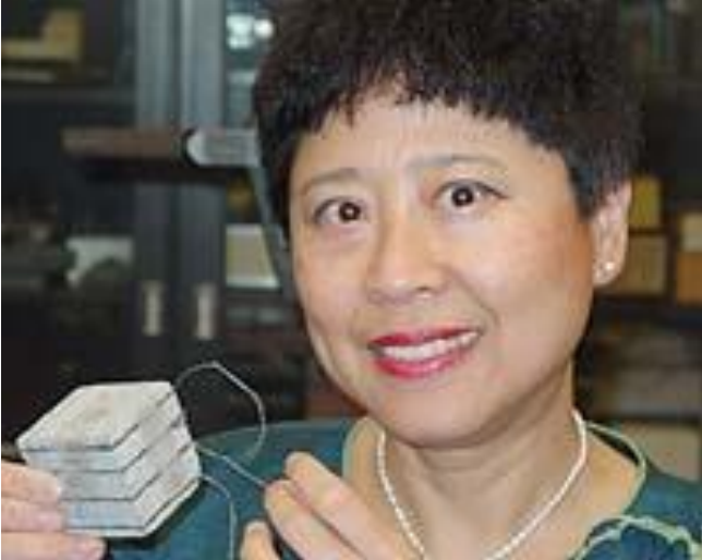
Figure 6. A sample of smart concrete using electrical properties as an ideal sensor of stress, weight and vibration.
