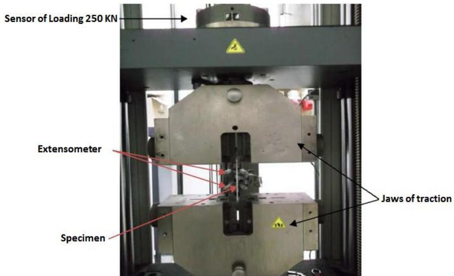
**Figure 4.** Universal machine of Zwick/Roell type 250KN.
