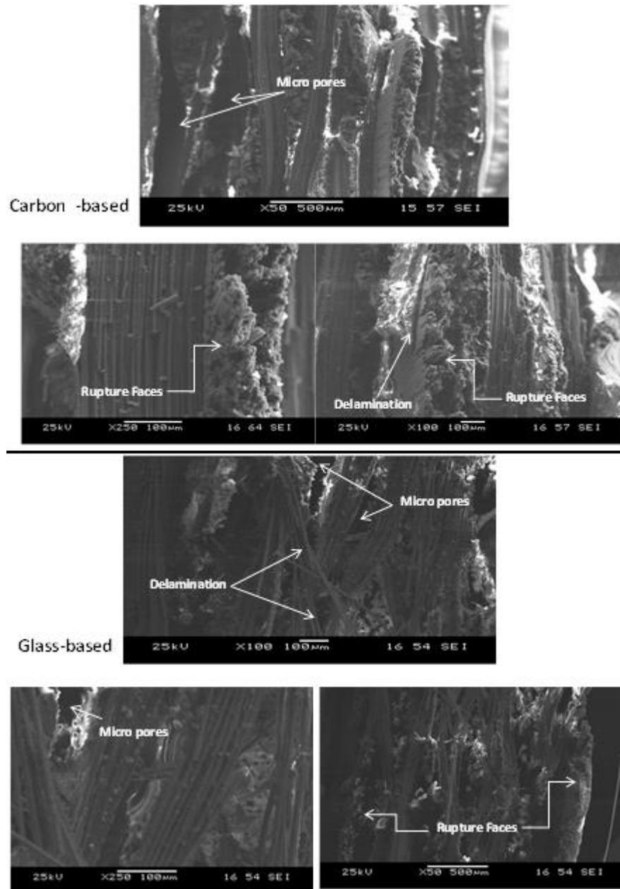
**Figure 10.** SEM micrographic of laminated after failure.
