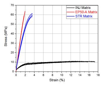
Figure 1. Tensile behavior of used resins.
