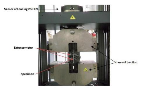
Figure 4. Universal machine of Zwick/Roell type 250KN.
