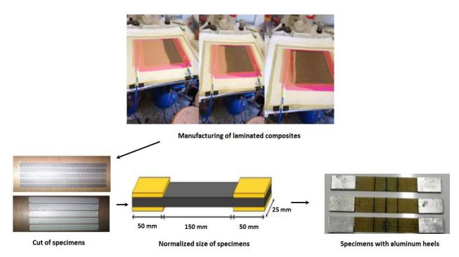
Figure 3. Specimen preparation and fabrication.
