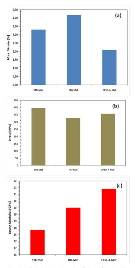
**Figure 6.** Mechanical properties of Glass-based laminates (a) Max. Strain (b) Stress (c) Young modulus
