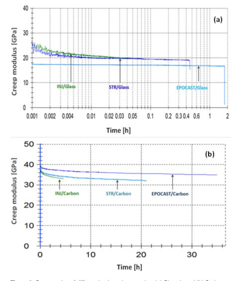
Figure 9. Creep testing of different laminated composites (a) Glass-based (b) Carbon-based
