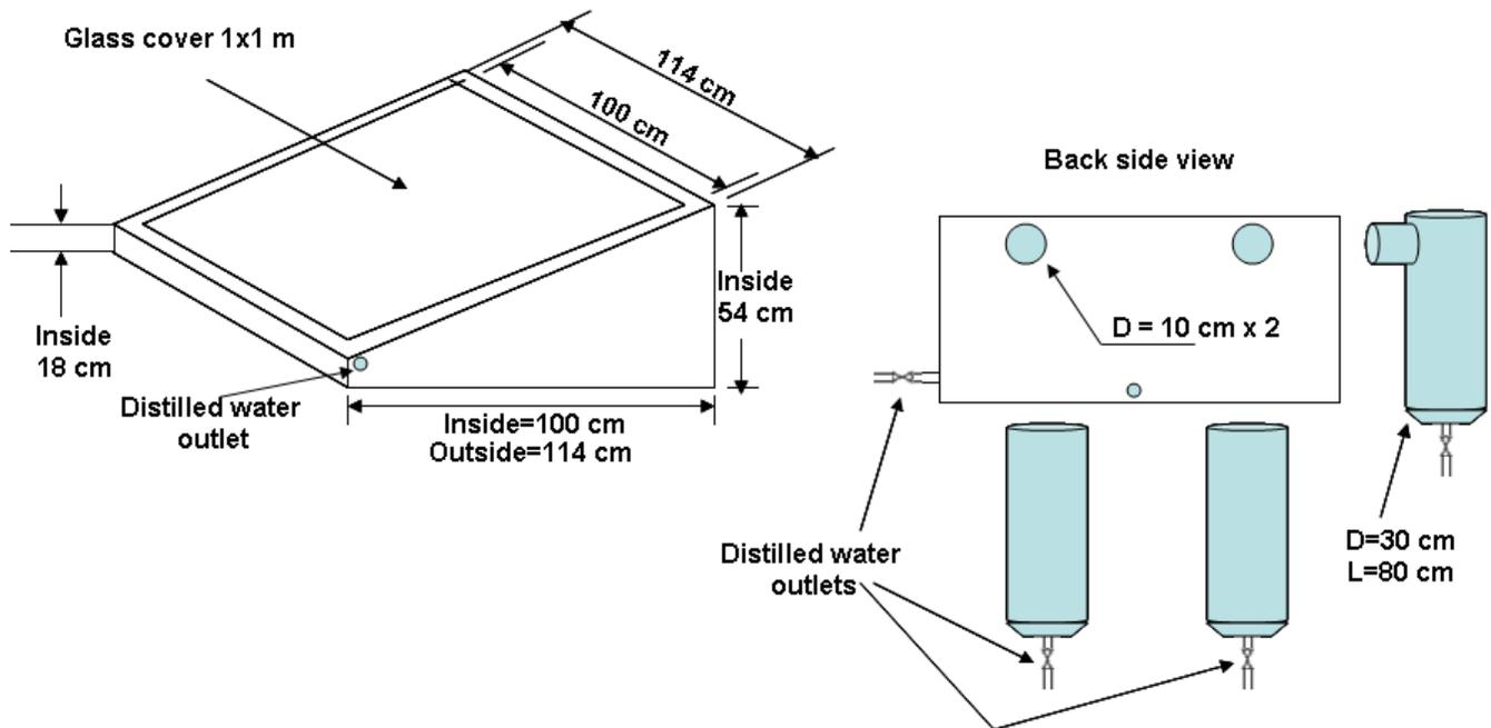
Figure 2. Schematic Diagram of Solar still linked to passive condensers by single connection.
