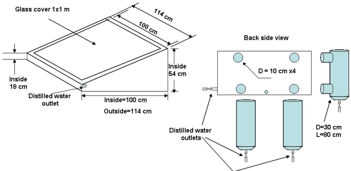
Figure 3. Schematic Diagram of Solar still linked to passive condensers by double connections.
