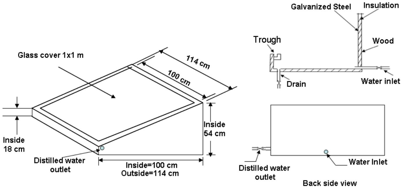
Figure 1. Schematic diagram of conventional solar still.
