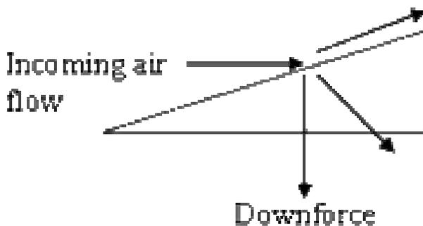
Figure 11. Downforce created due to incoming force of air.
