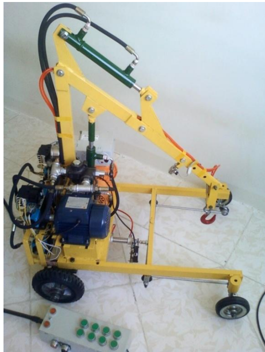
Figure 10. Steer-by-switch system mounted on a wire remote control crane.
