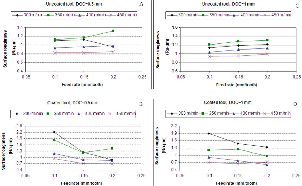
**Figure 4.** Change in surface roughness with respect to the feed rate.
