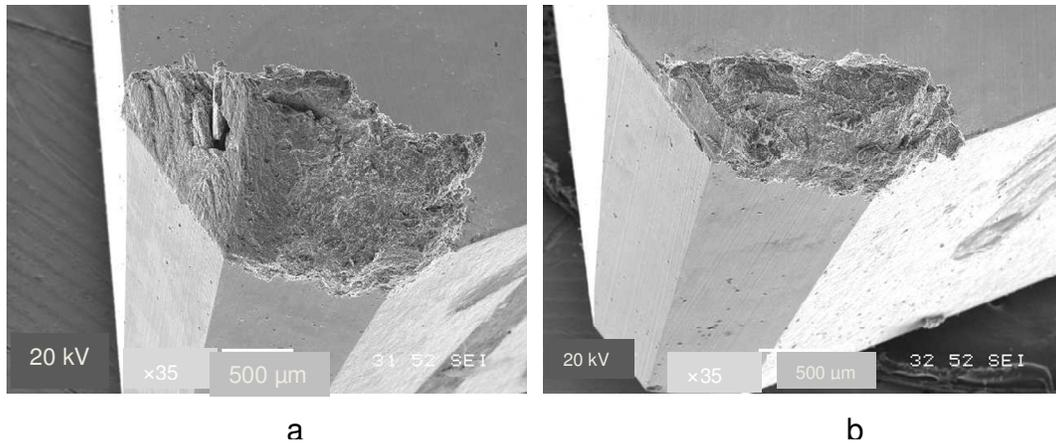
**Figure 5.** Built-up edge formation on the uncoated tool a) cutting speed of 300 m/min, feed rate = 0.1 mm/tooth and DOC= 1 mm, b) cutting speed of 450 m/min, feed rate = 0.1 mm/tooth and DOC= 1mm ( $\times 35$ ).
