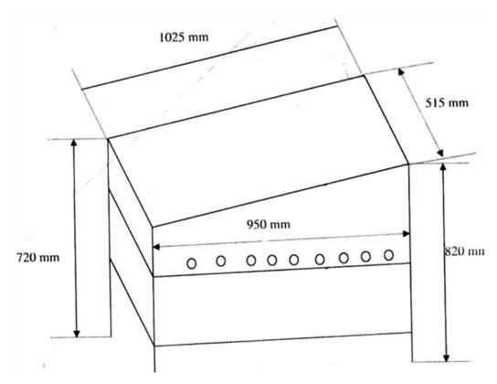
**Figure 1.** A schematic diagram of the passive solar dryer (National Centre of Energy Research and Development (NCERD), University of Nigeria, Nsukka).
