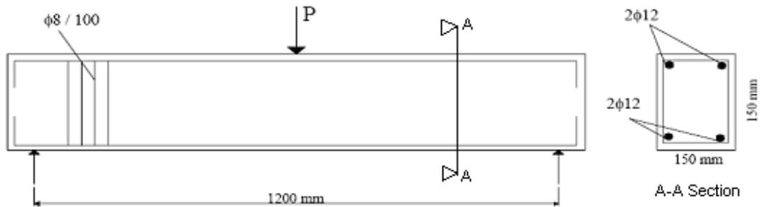
Figure 1. Reinforcement detail of control specimen.
