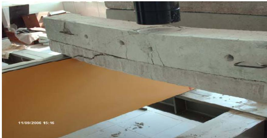
**Figure 14.** Picture of strengthened specimen after failure.
