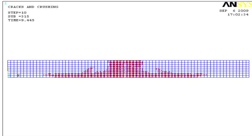
Figure 10. Cracks of control specimen at failure.
