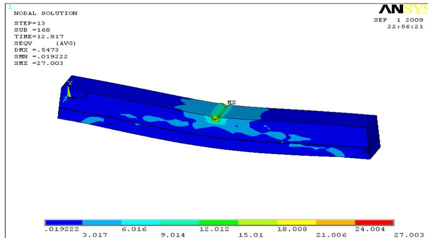
**Figure 13.** Stress of strengthened specimen at the failure.
