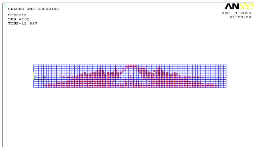
Figure 12. Cracks of strengthened specimen at failure.
