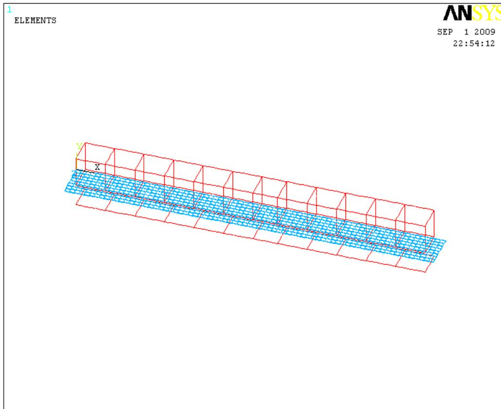
**Figure 7.** Reinforcements, stirrups and epoxy modelling of strengthened specimen.
