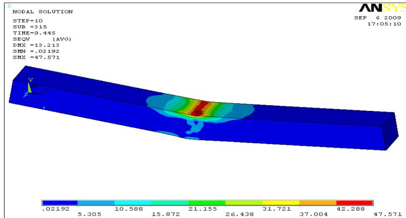
Figure 11. Stress of control specimen at failure.
