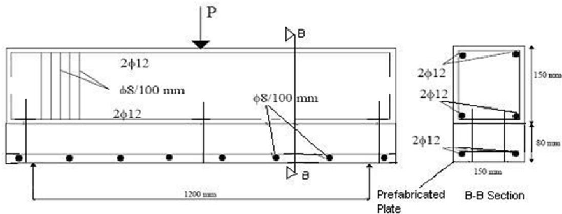
Figure 2. Reinforcement detail of strengthened specimen.
