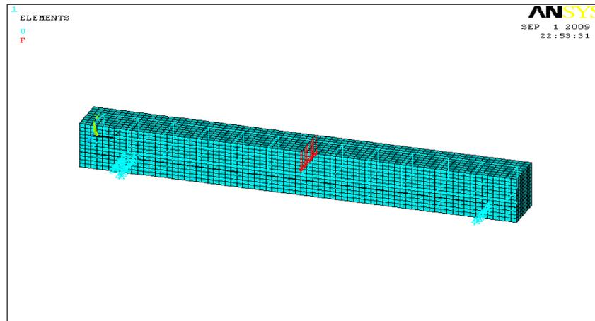
Figure 9. Loads and supports of strengthened specimen.
