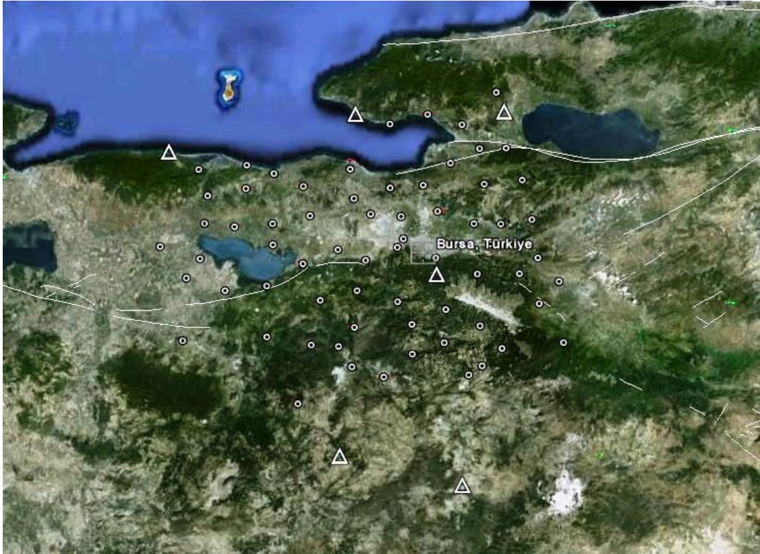
Figure 3. Active faults around the Bursa basin. The solid white lines display the active faults (the satellite image obtained from google earth).
