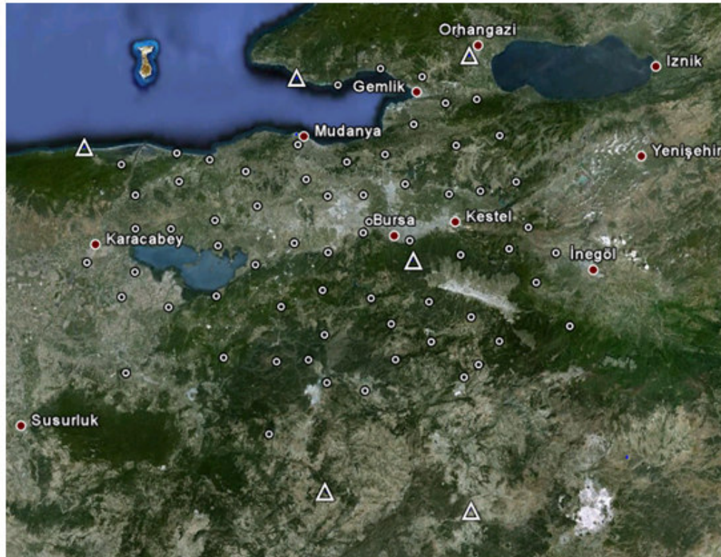
Figure 1. The basic GPS network in BMA. The triangles represent TUTGA points while the dotted circles represent the other basic network points (The satellite image obtained from google earth).
