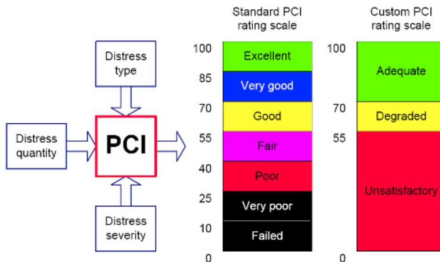
Figure 1. Pavement quality – PCI (Micropaver 5.3 Manual).
