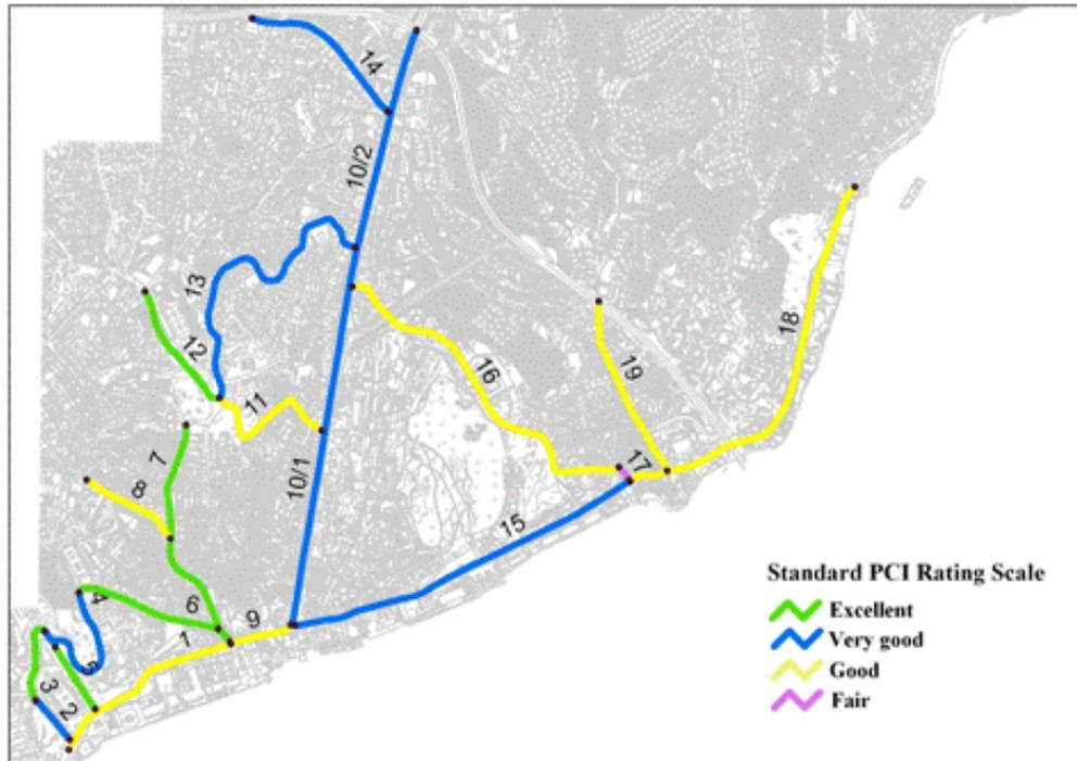
**Figure 2.** Sections situation for standard PCI rating scale.
