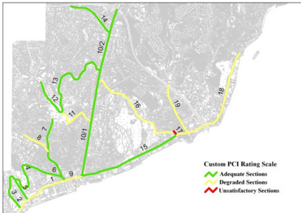
Figure 3. Sections situation for custom PCI rating scale.
