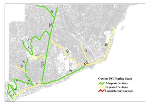
Figure 3. Sections situation for custom PCI rating scale.
