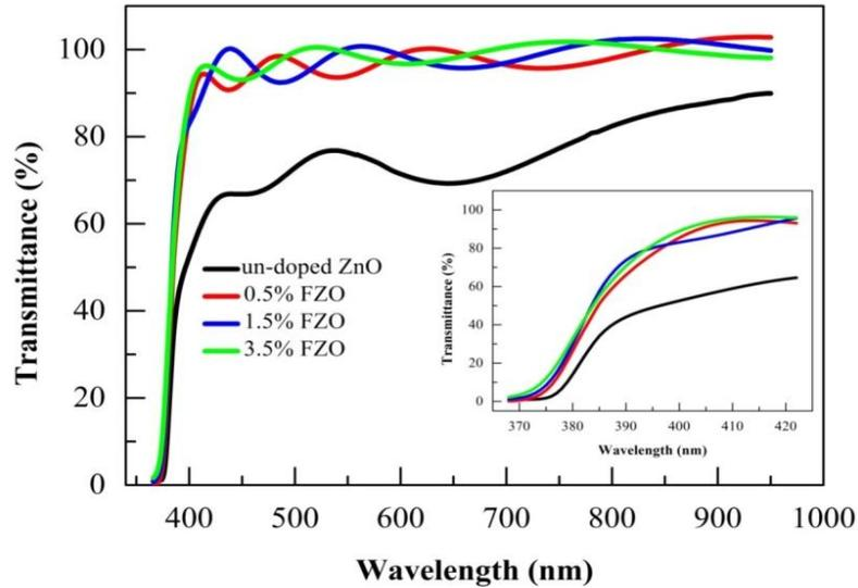
**Figure 3.** Optical transmittance spectra of un-doped and various F-doped ZnO films and inset figure shows the transmittance spectra at short wavelengths.
