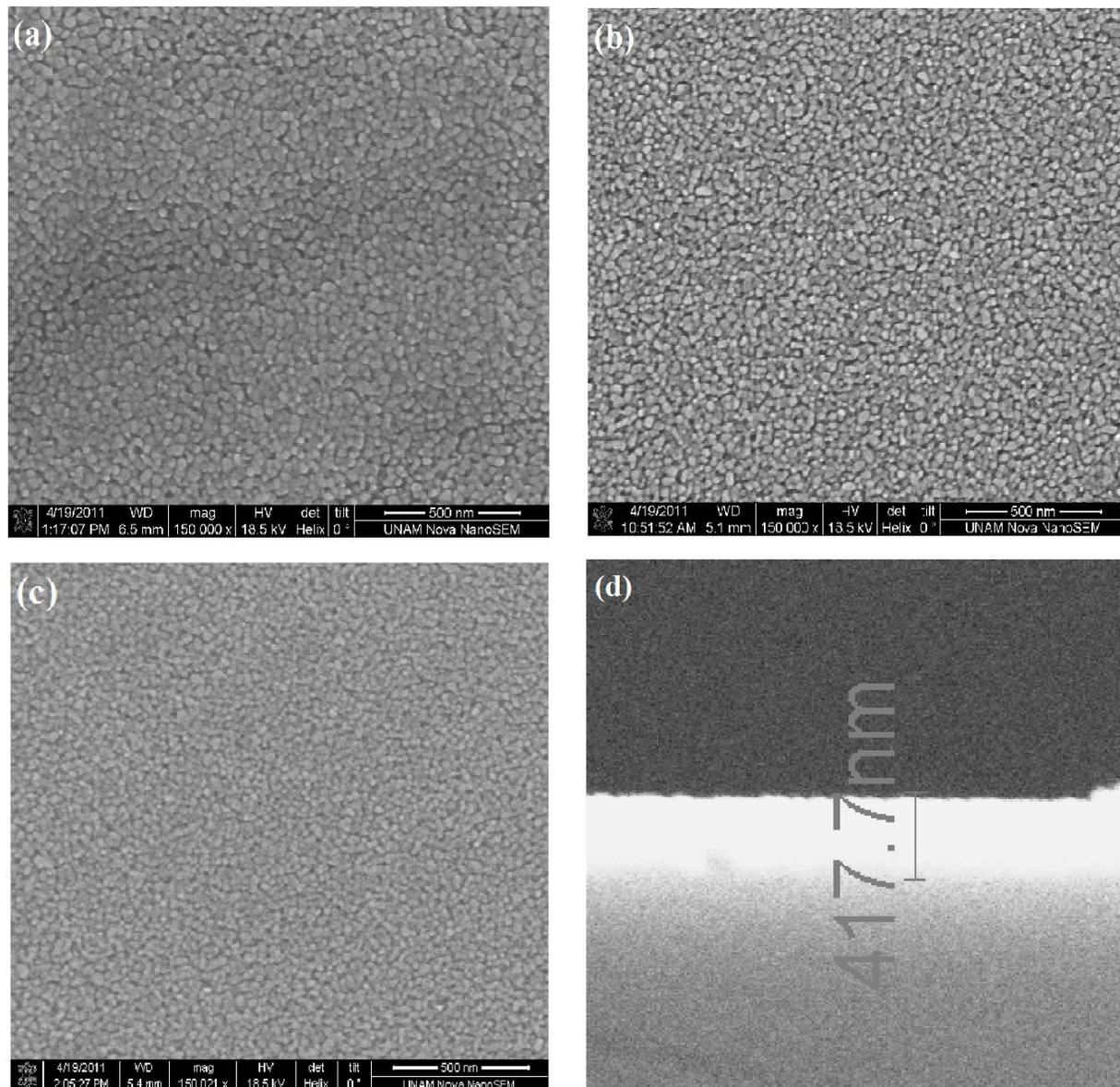
**Figure 2.** SEM micrograph of ZnO films with different fluorine concentrations: (a) F<sub>0.5</sub>ZO; (b) F<sub>1.5</sub>ZO; (c) F<sub>3.5</sub>ZO; (d) cross sectional SEM image for average film thickness (0.5% mole).
