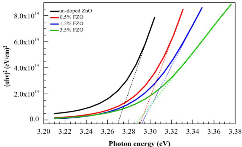
**Figure 4.** Plot of  $(\alpha h\nu)^2$  versus photon energy for F-doped ZnO thin films.
