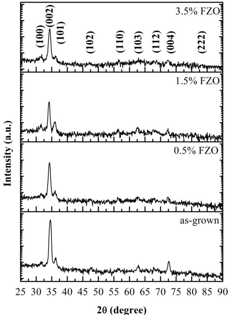
Figure 1. XRD patterns of ZnO thin films with different fluorine contents.
