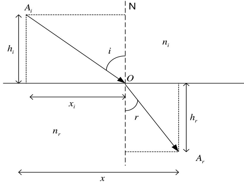
Figure 1. Refraction of light.
