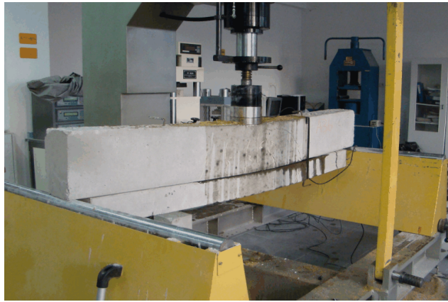
Figure 3. The loading of the strengthened beam.
