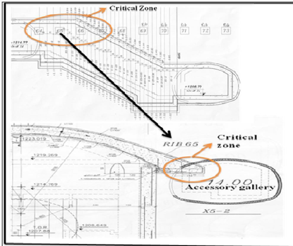
Figure 1. Cross section of metro tunnel showing critical zone of station and access galleries.
