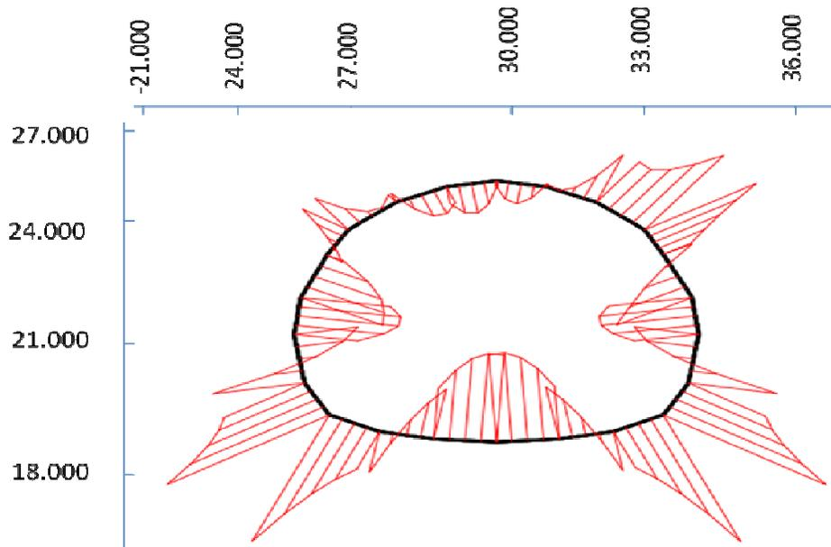
(E) Vertical displacements (Extreme vertical displacement  $71.97 \times 10^{-3}$  m).
