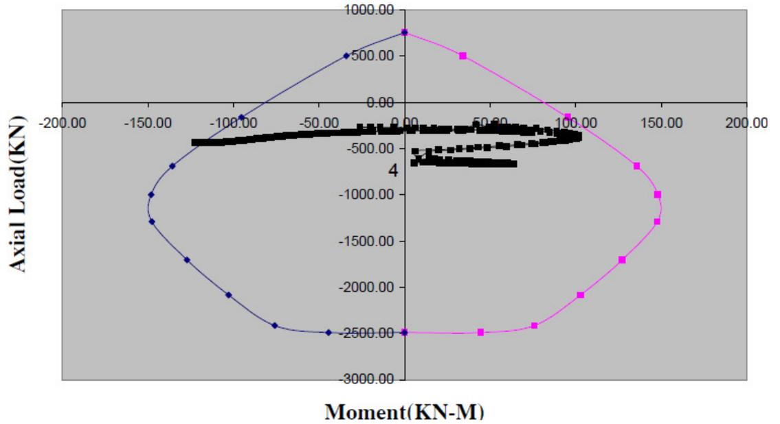
Figure 2. Interaction lattice frame (shotcrete =30 cm, bar = 25).
