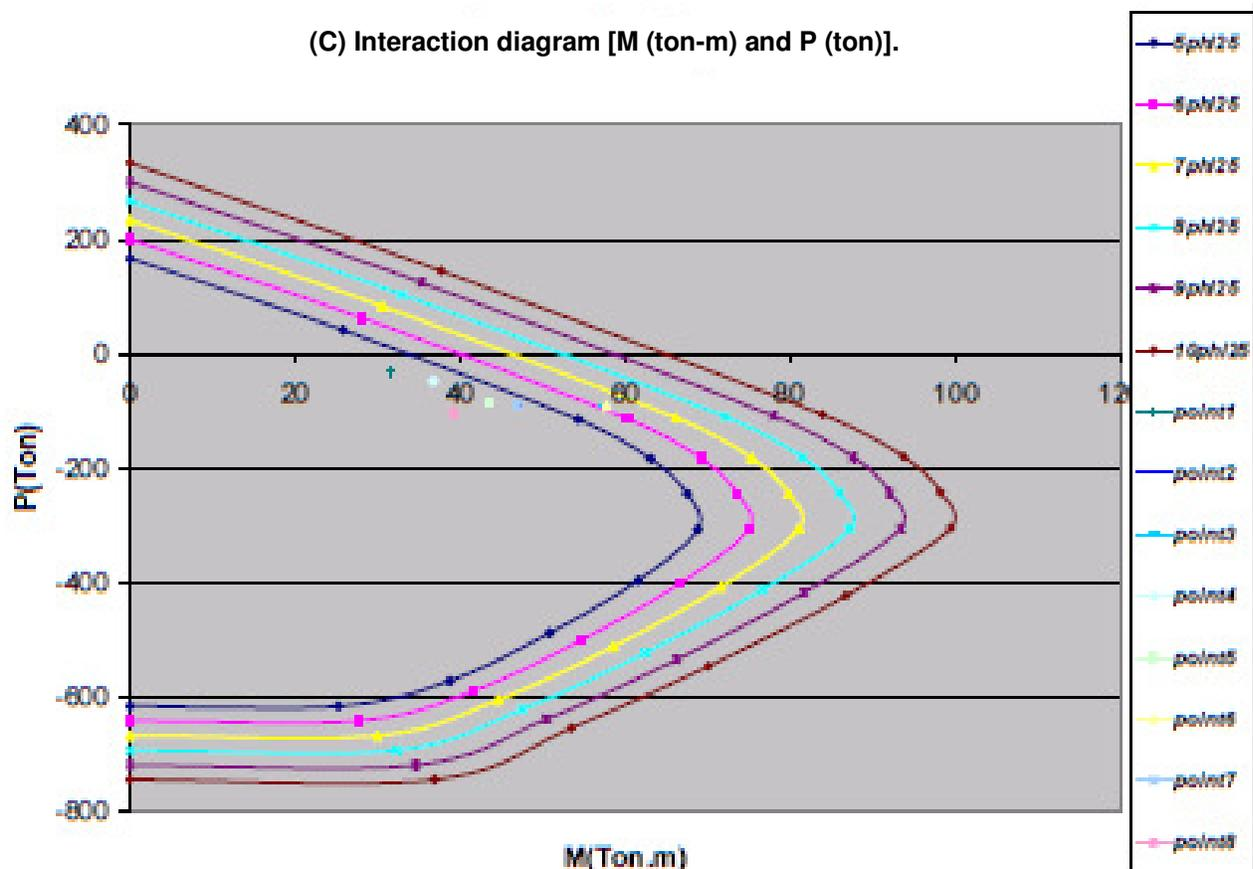
**Figure 8.** Interaction diagrams, (A and B) for 20 m overburden, and (C) for 30 m overburden based on M (ton-m) and P (ton) of tunnel with 20 m and 30 m overburden.
