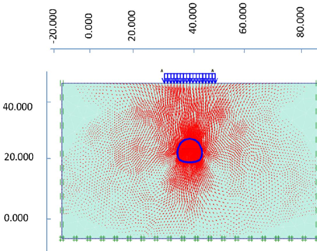
(C) Horizontal displacement (Extreme horizontal displacement  $10.30 \times 10^{-3}$  m).
