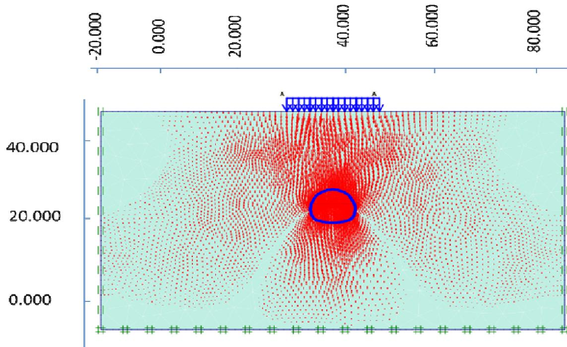
Figure 4. PLAXIS outputs for tunnel with 20 m overburden, (A) Typical mesh, (B) Total displacement, (C) Horizontal displacement, (D) Bending moment, and (E) Vertical displacement.
