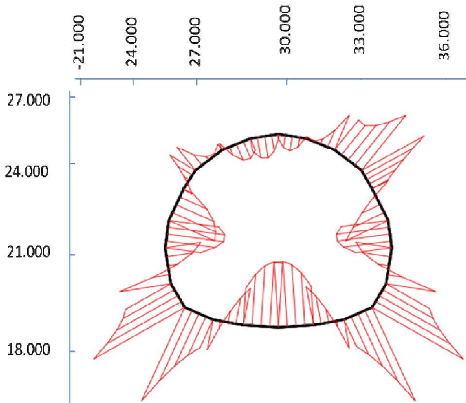
(D) Total displacements (Extreme total displacement  $71.97 \times 10^{-3}$  m).
