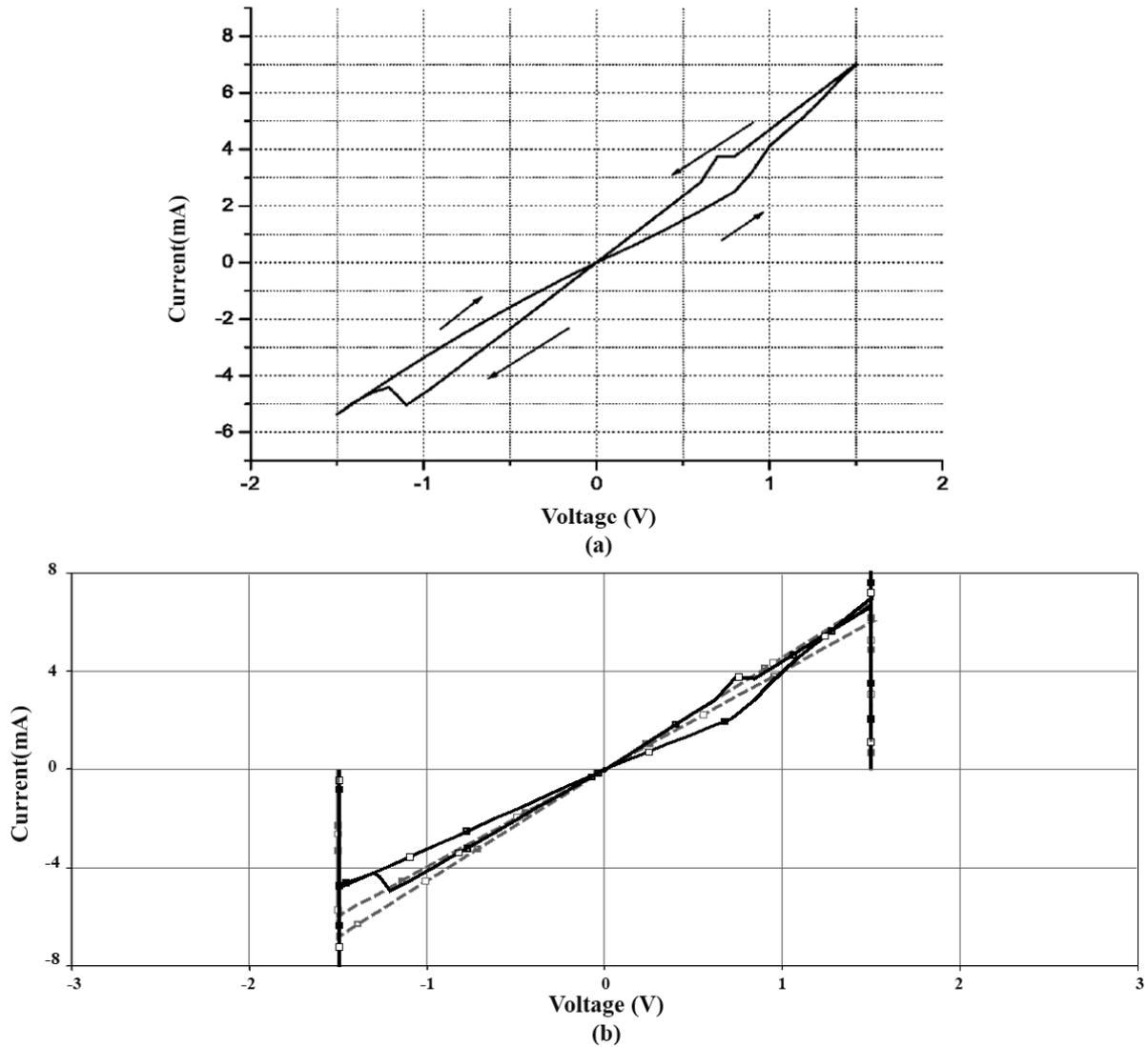
**Figure 8.** (a)  $I$ - $V$  characteristic of the ITO/aluminum stack which shows hysteresis behavior. Figure source: Lüssem, (2006). (b) The simulation result curves by the use of the LHM (dashed line) and GHM (solid line). For achieving the LHM output the forward and reverse slope values are specified by utilizing two different resistors ( $250 \Omega$  and  $219 \Omega$  respectively).
