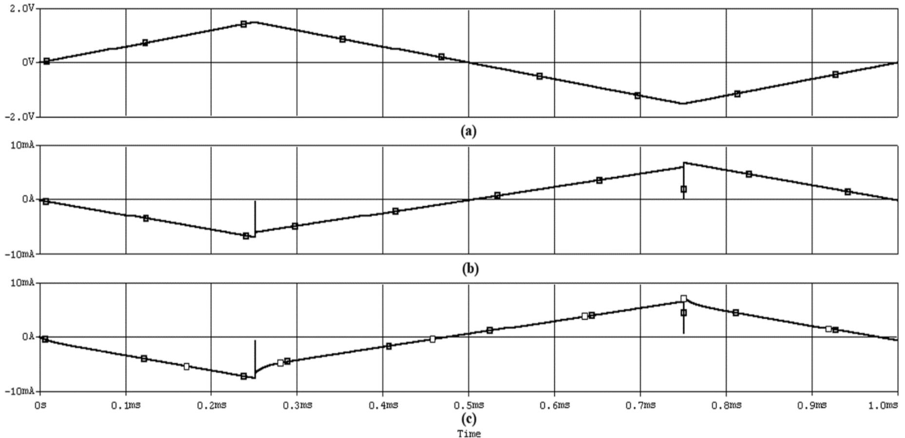
**Figure 10.** The effect of using integrator circuit in the proposed circuit for modeling the Figure 7  $I/V$  curve. (a) Applied voltage. (b) Current curve without exploiting the integrator circuit. (c) Current curve after modification and with exploitation of the integrator circuit. The applied characteristics are:  $C_f=100$  nF and  $R_f=0.1$  k $\Omega$ .
