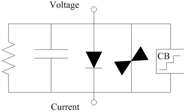
**Figure 1.** Two-terminal UDM. The main features of this model are capacitance, resistance, thermionic emission, NDR, and coulomb blockade.
