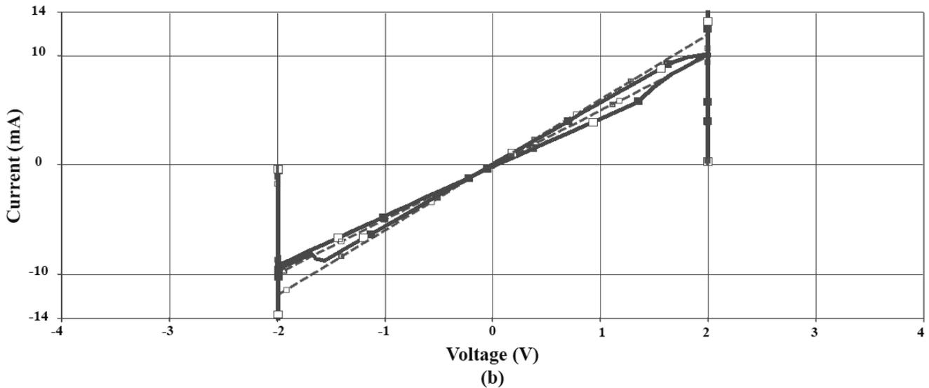
**Figure 7.** (a) *I-V* characteristic of the ZnO/aluminum stack which shows hysteresis behavior. Figure source:Lüssem (2006). (b) The simulation result curves by the use of the LHM (dashed line) and GHM (solid line). For achieving the LHM output the forward and reverse slope values are specified by utilizing two different resistors (166 Ω and 200 Ω respectively).
