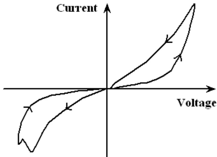
**Figure 4.** A generic  $I$ - $V$  curve for a typical molecular hysteresis switch. Figure source: Rose and Stan (2007).
