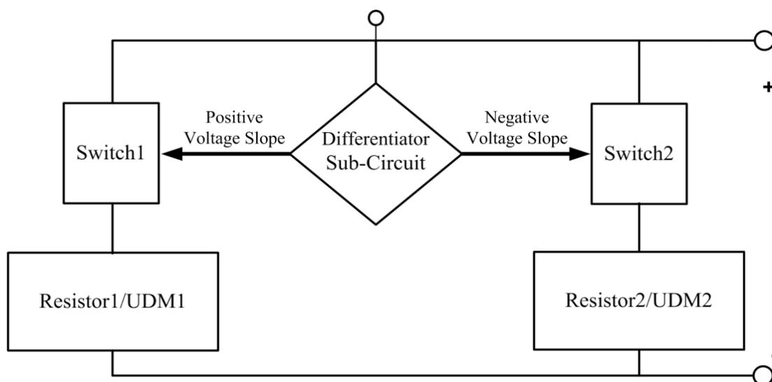
**Figure 5.** Block diagram for the proposed behavioral model. The differentiator sub-circuit selects one of the resistors/UDM modules. And the selected resistors/UDM modules generate appropriate current.
