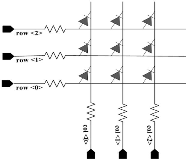
**Figure 2.** Equivalent circuit schematic of a crossbar technology.
