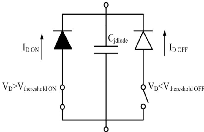
**Figure 3.** A device model for crossbar technology. Figure source: Ziegler and Stan (2003). Two diodes are used for showing the on-state and off-state of a cross bar junction.
