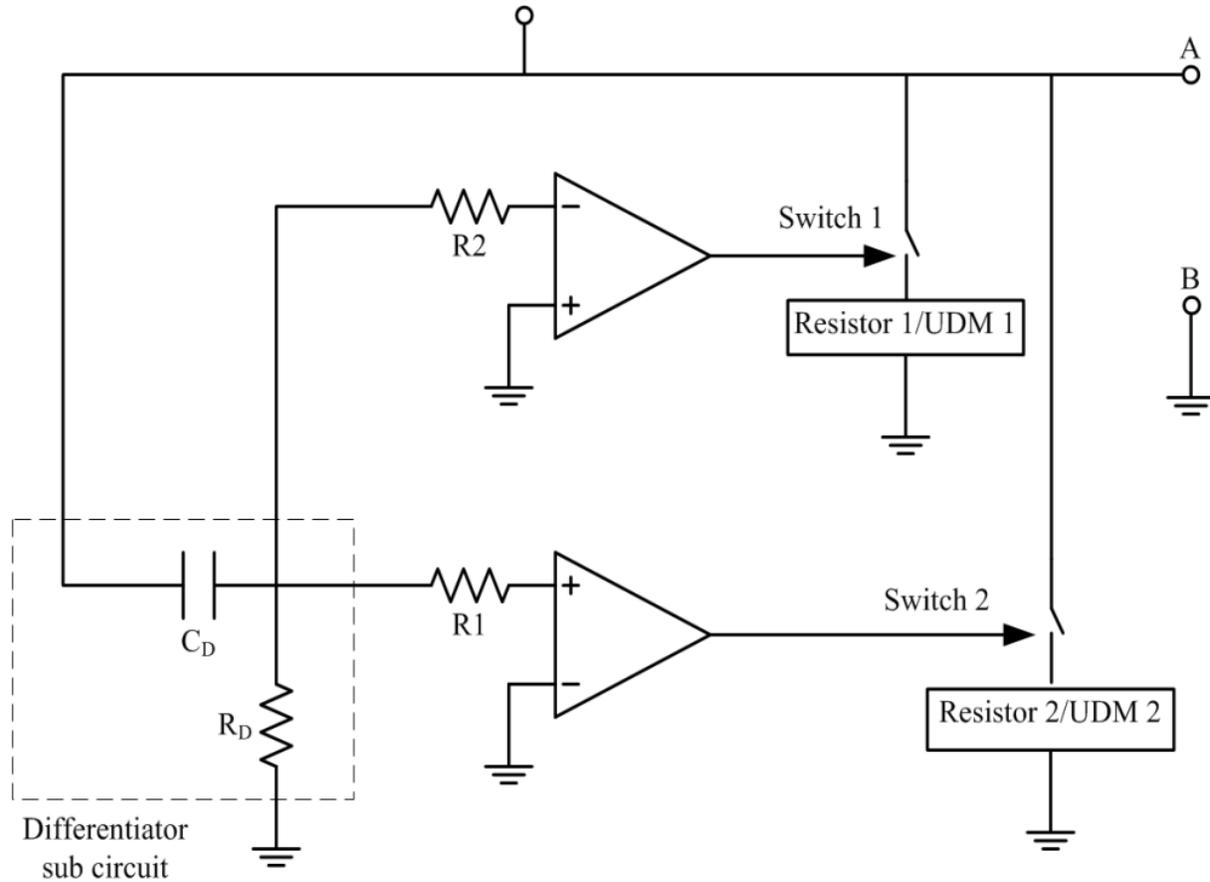
**Figure 6.** The proposed circuit model for imitating hysteresis behavior. This model consists of a differentiator sub-circuit, two switches and two resistor/UDM modules.
