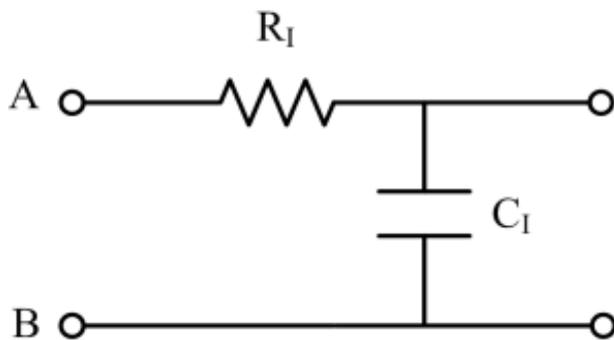
**Figure 9.** Applying simple integrator circuit helps to achieve continuous curves in the output.
