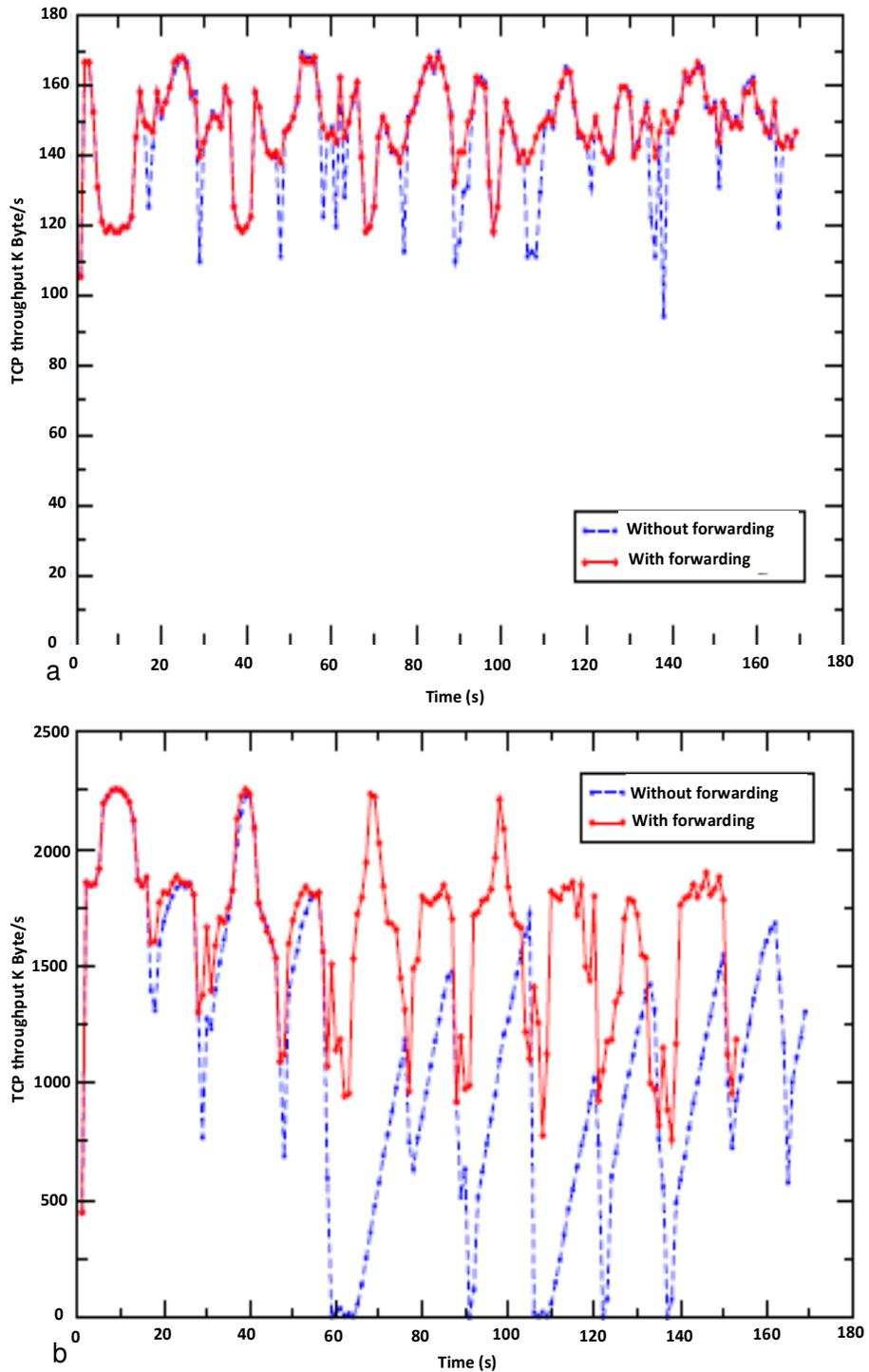
**Figure 6.** a. TCP throughput with and without with and without forwarding (2 Mbps radio link rate); b, TCP throughput forwarding (20 Mbps radio link rate).
