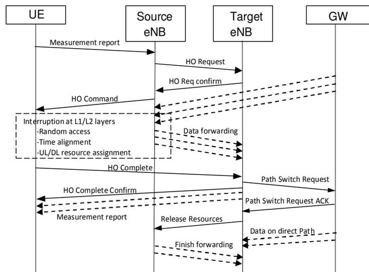
Figure 5. Message chart of the LTE handover procedure (Racz et al., 2007).
