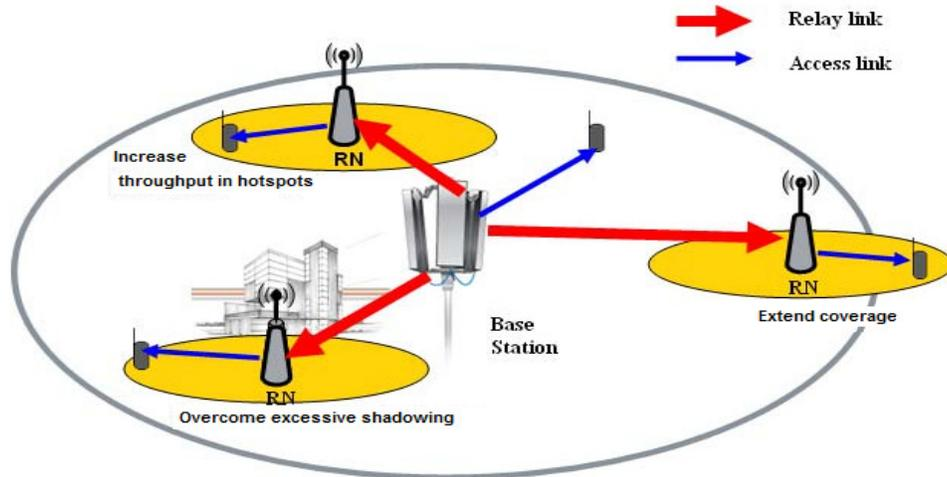
**Figure 7.** Example scenarios for the deployment of RNs in LTE network.
