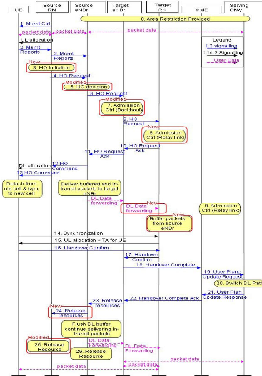
Figure 9. Handover in LTE supporting decentralized relaying.
