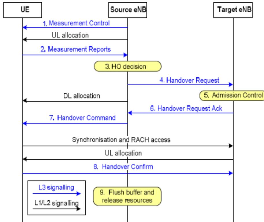
Figure 3. Handover process in LTE network (3GPPTS 36.300 V.870, 2008).
