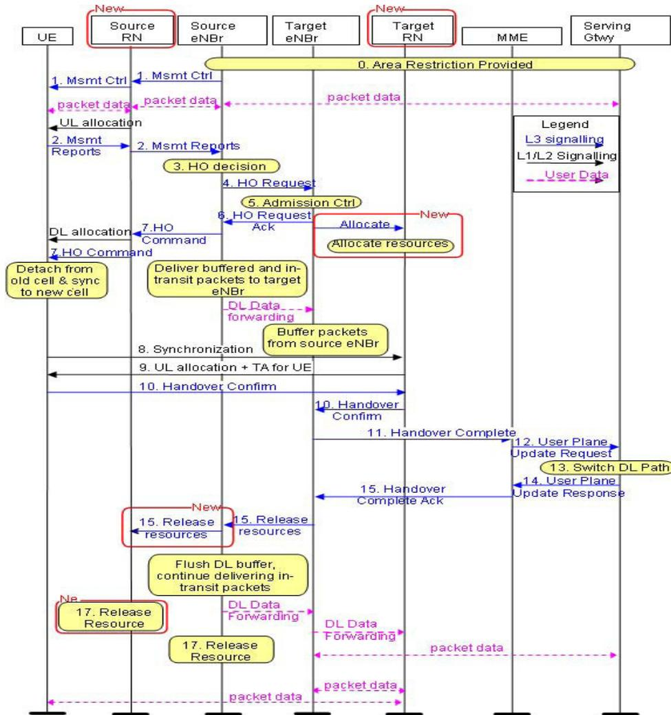
Figure 8. Handover in LTE supporting centralized relaying.
