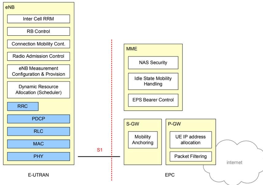
Figure 2. Functional division between E-UTRAN and EPC (3GPP TS 36.300 V8.6.0, 2008).
