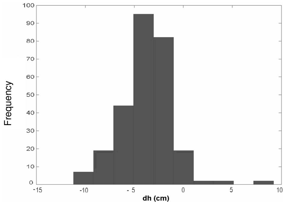
**Figure 5.** Frequency histogram of differences in heights obtained for the same details with respect to wall and classical traverse techniques.
