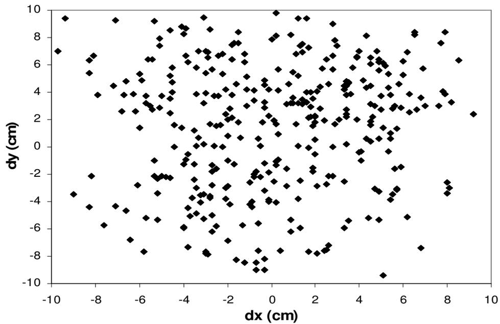
**Figure 4.** Distribution of differences in coordinates (dx and dy) obtained for the same details with respect to wall and classic traverse techniques.
