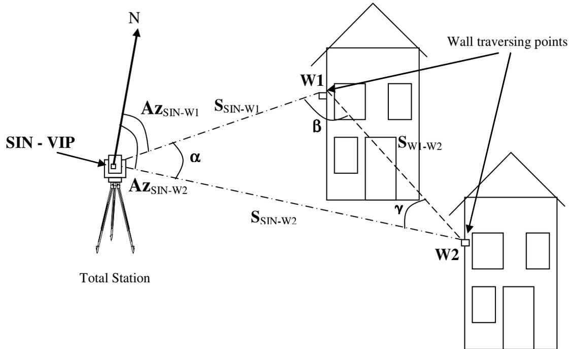
**Figure 1.** Determination of SIN (VIP) by wall traverse technique.
