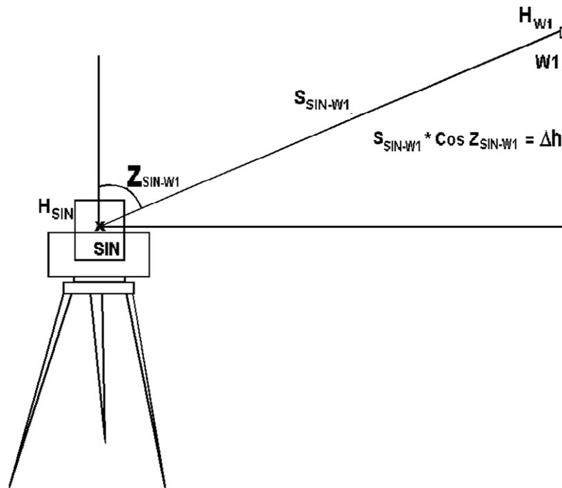
Figure 2. Determination of height of a SIN by the help of wall survey point.
