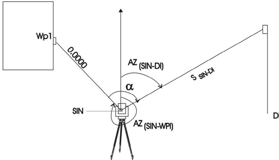
Figure 3. Detail measurement by wall traverse.
