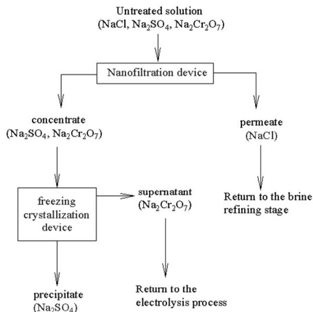
**Figure 3.** The process flow diagram.
