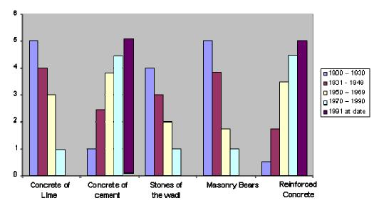
**Figure 4.** Evolution of the materials and processes of construction.
