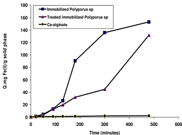
**Figure 3.** Biosorption capability of immobilized *P. squamosus* and plain Ca-alginate for Fe(II) ions in refinery effluent
