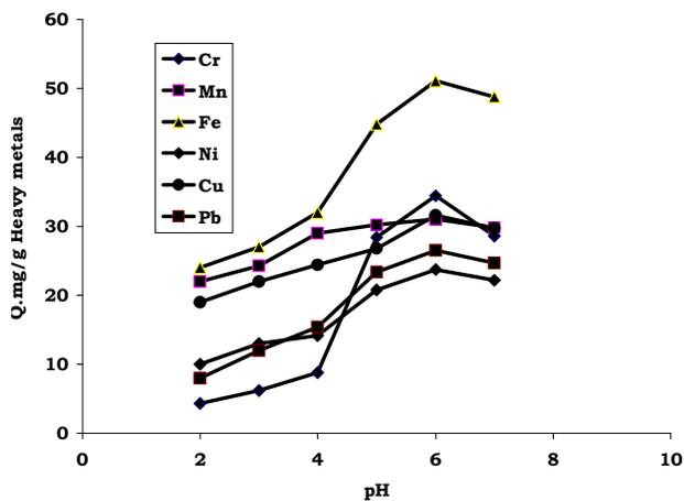
Figure 8. The effect of solution pH on the biosorption of Heavy metals non-treated effluent by immobilized *P. squamosus*.
