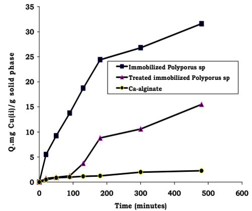
**Figure 5.** Biosorption capability of immobilized *P. squamosus* and plain Ca-alginate for Cu(II) ions in refinery effluent
