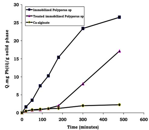
**Figure 6.** Biosorption capability of immobilized *P. squamosus* and plain Ca-alginate for Pb(II) ions in refinery
