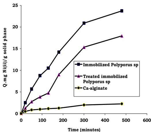
**Figure 4.** Biosorption capability of immobilized *P. squamosus* and plain Ca-alginate for Ni(II) ions in refinery effluent
