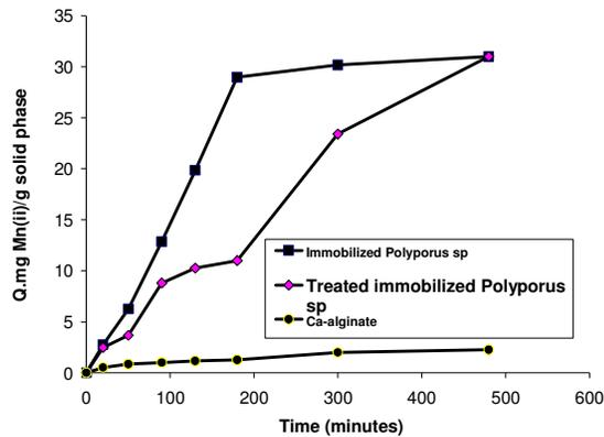
**Figure 2.** Biosorption capability of immobilized *P. Squamosus* and plain Ca-alginate for Mn(II) ions in refinery effluent
