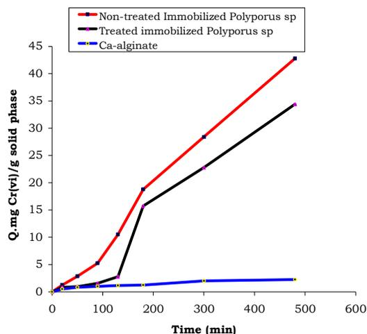
**Figure 1.** Biosorption capability of immobilized *P. squamosus* and plain Ca-alginate for Cr(VI) ions in refinery effluent.
