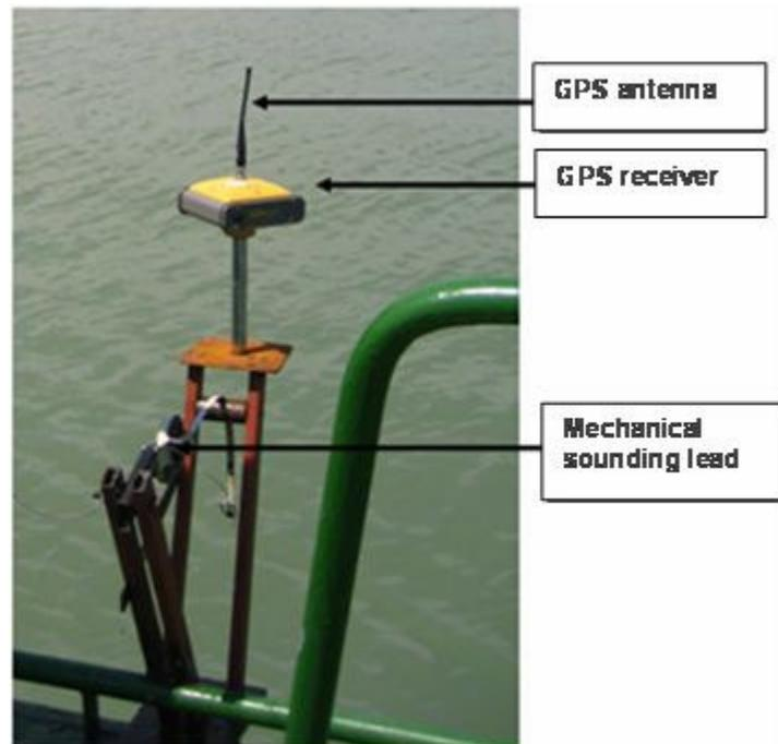
Figure 2. Mechanical sounding lead.
