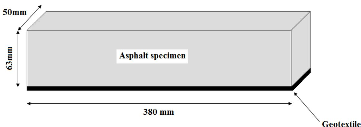
Figure 1. The specimen dimensions and the location of geotextile.
