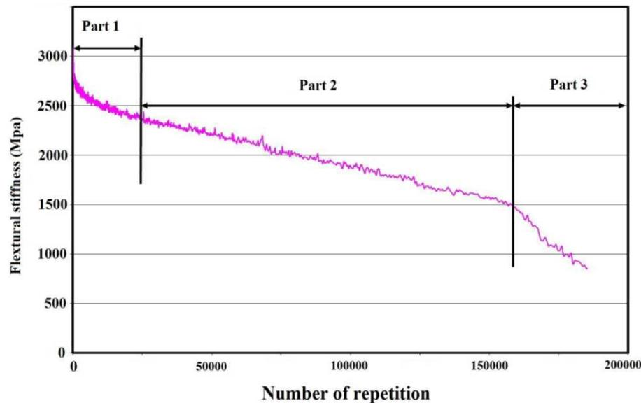
**Figure 2.** Flexural stiffness diagram against the repetition of loading.
