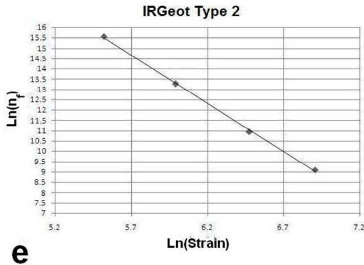
Figure 5. Fatigue life against strain level of five types of specimens.
