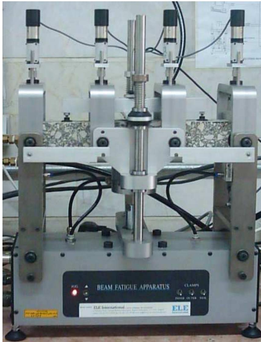
**Figure 3.** The general view of the bending beam fatigue apparatus.
