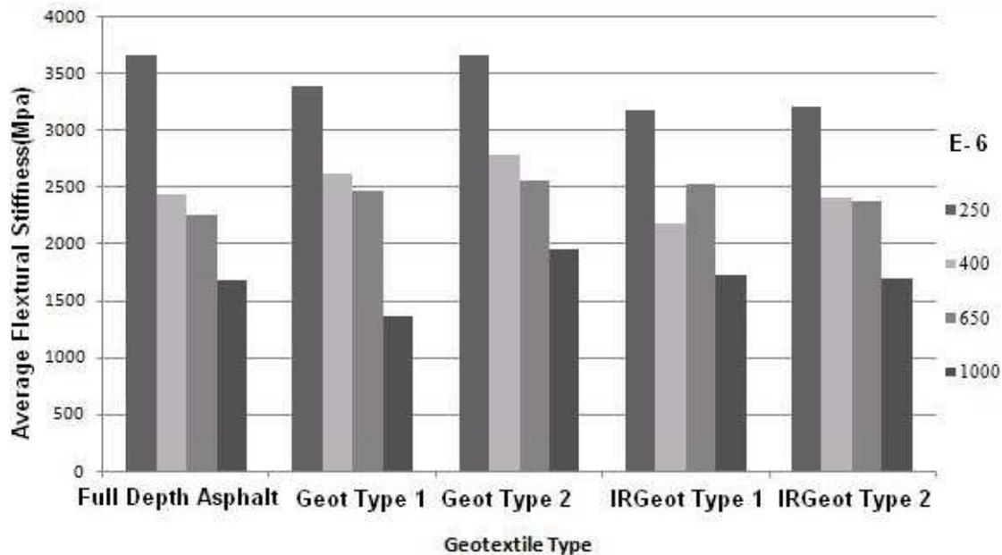
Figure 6. The average flexural stiffness versus the specimen's types.
