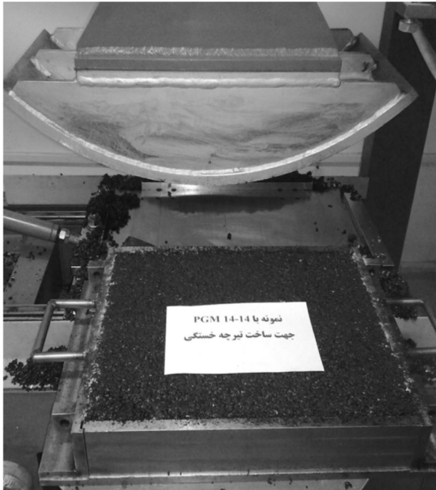
**Figure 4.** One of the slabs made from the HMA and geotextile.
