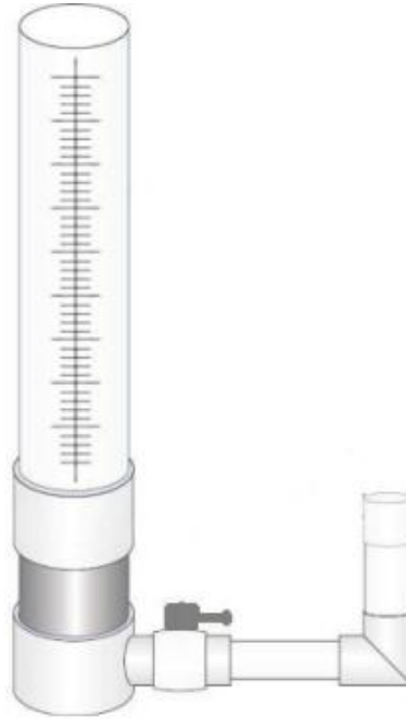
Figure 2. Falling head method kit for permeability coefficient measurement.
