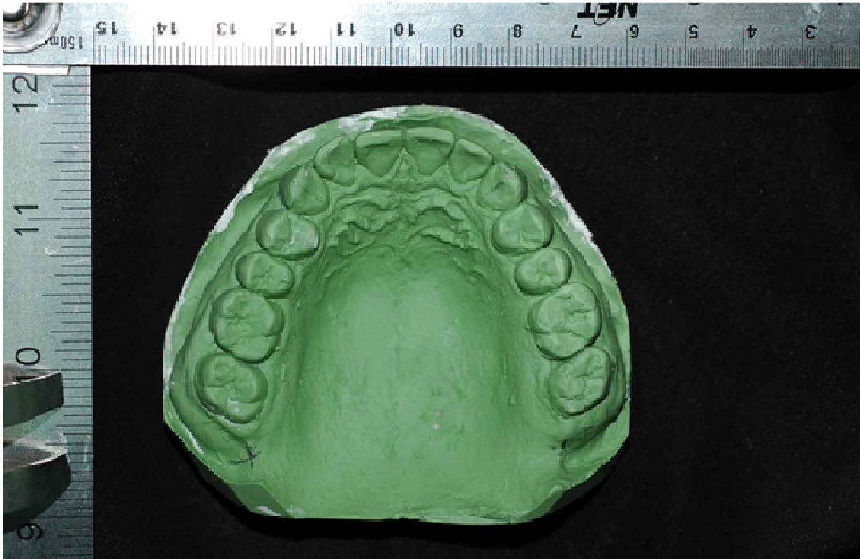
Figure 1. Standardized position of the cast when its digital image was captured. Two metal rulers were positioned on a plane parallel to the occlusal plane for calibration of the measurements.
