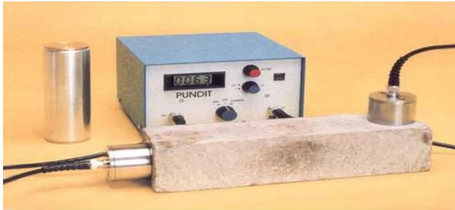
**Figure 1.** Pulse velocity testing equipment (PUNDIT).
