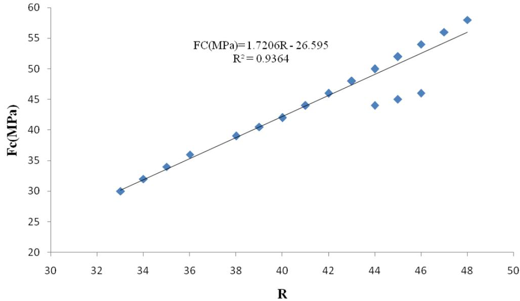
Figure 5. Rebound number/compressive strength calibration curve.
