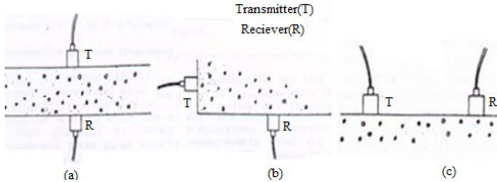
Figure 2. Direct (a), Semi-direct (b) Indirect (surface) transmission (c).
