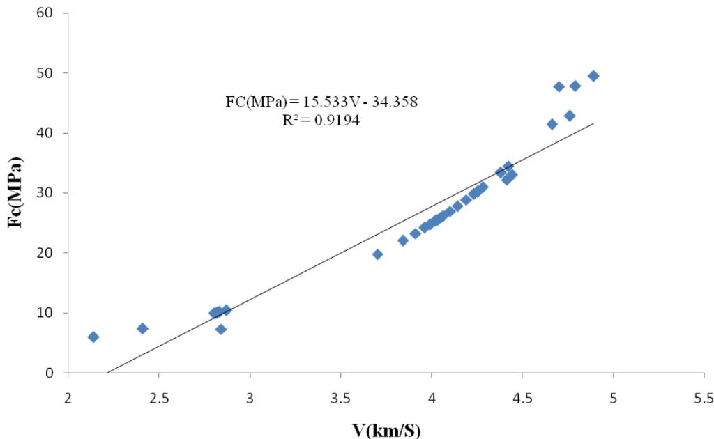
**Figure 6.** Ultrasonic Pulse Velocity (UPV)/compressive strength calibration curve.
