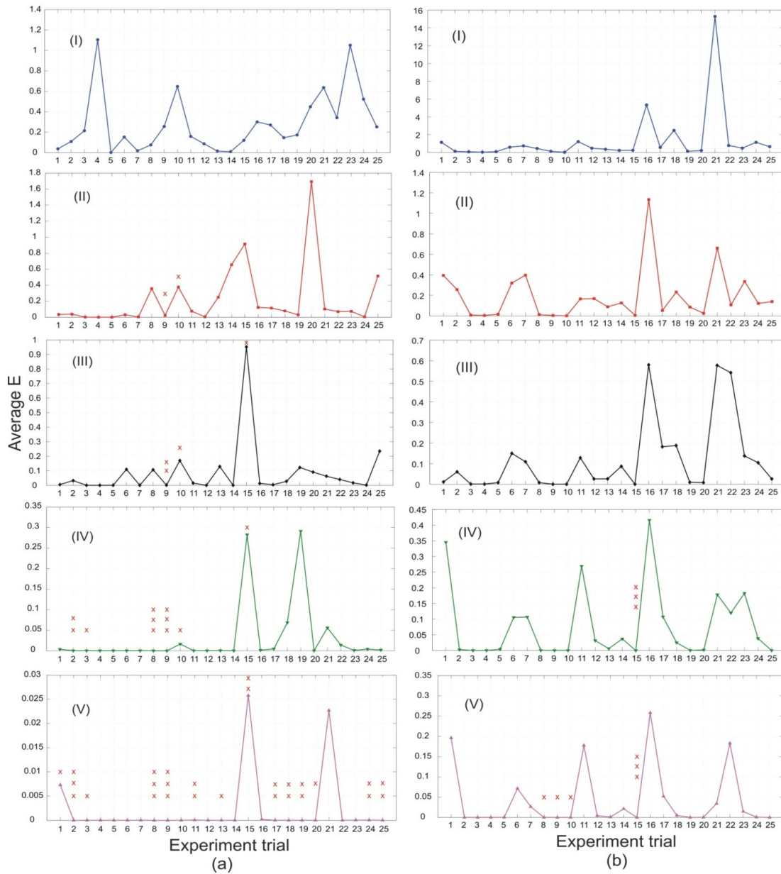
Figure 1. The performance of IHSA: (a), Rosenbrock function; (b), Wood-Colville function.
