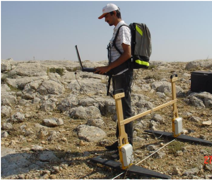
Figure 4. Ramac/GPR CU-II with 100 MHz antennas (transmitter and receiver) at starting point of Haymana profile.
