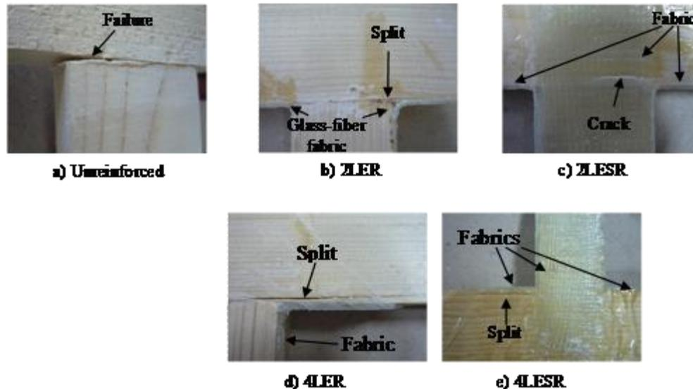
Figure 8. Photography of failed specimens.
