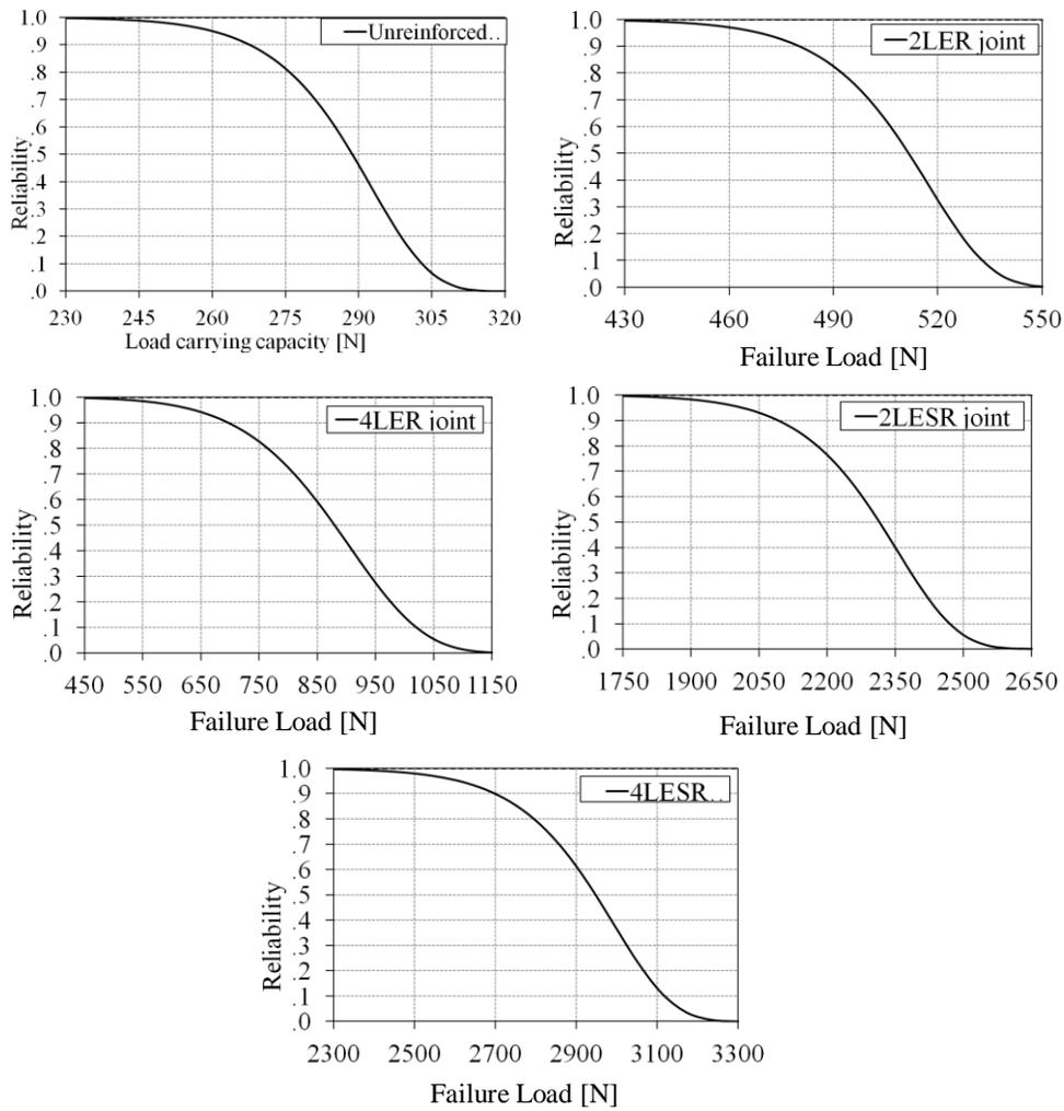
Figure 6. Weibull reliability distribution for failure load.
