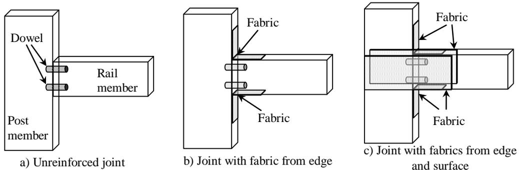
**Figure 3.** The configuration of T-type joints.
