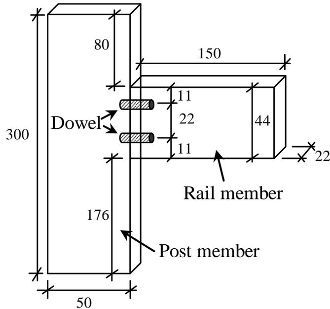
**Figure 2.** Typical configuration of the specimens used in the test (Dimensions in mm).
