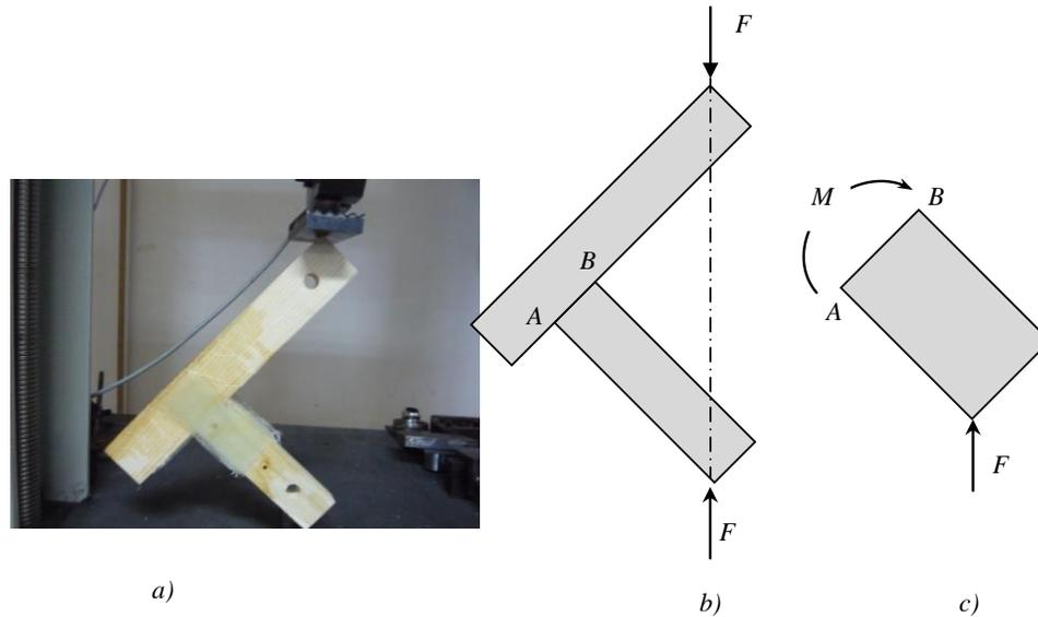
**Figure 4.** Load specimen and loading type.
