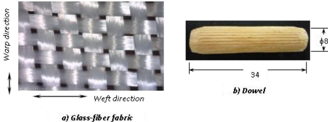
Figure 1. Fastener materials (Dimensions in mm).
