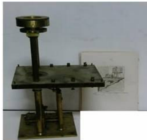
Figure 20. Myograph of Helmholtz.
