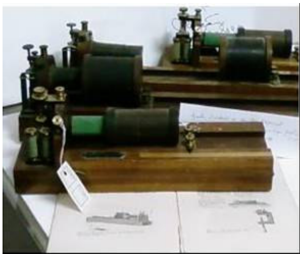
Figure 19. Du Bois Raymond induction instruments.
