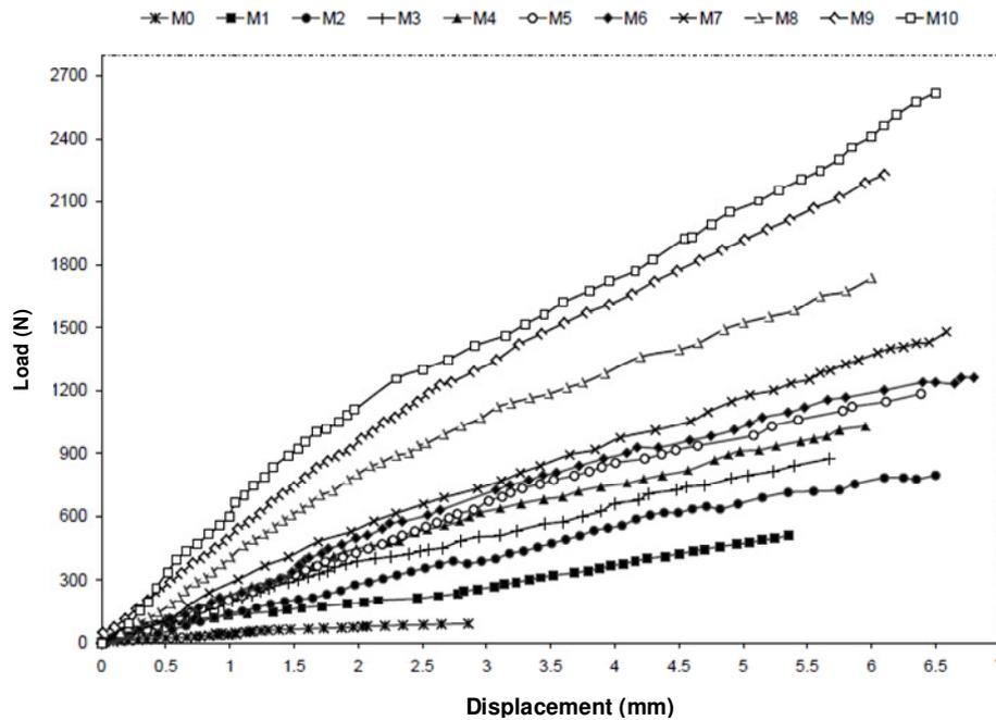
**Figure 7.** Flexural load-displacement graphic, M0-unreinforced specimen.
