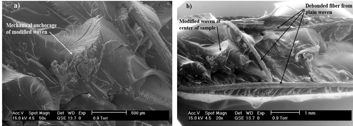
**Figure 6.** Mechanical anchorage a) Magnification of a knot b), Test specimen of group M4 with modified (MWHF) and (PWHF) plain henequen woven fabric.
