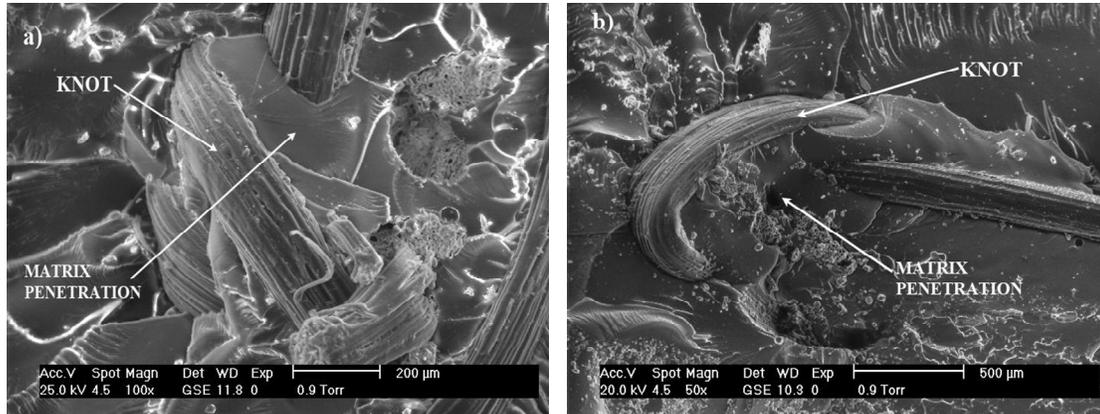
**Figure 4.** Matrix penetration inside knots in MWHF. (a) Tension test specimen, (b) Flexural test specimen.
