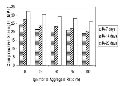
Figure 3. Effect of age, aggregate ratio on the compressive strength of IA concretes.
