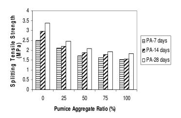
**Figure 5.** Effect of age, aggregate ratio on the splitting tensile strength of PA concretes.
