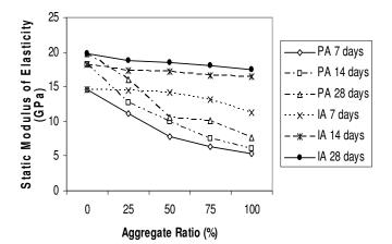
Figure 7. Static modulus of elasticity variation of PA, IA, and CGA
