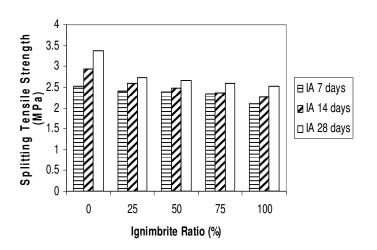
Figure 6. Effect of age, aggregate ratio on the splitting tensile strength of IA concretes.
