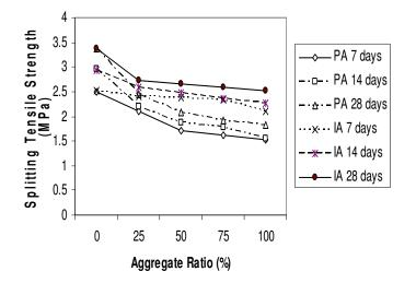
Figure 4. Splitting tensile strength variation of PA, IA, and CGA concretes for different aggregate ratios and ages.
