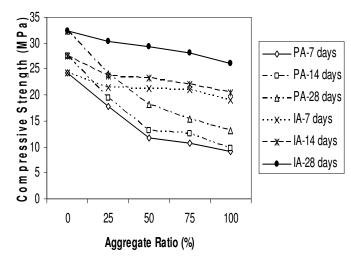
**Figure 1.** Compressive strength variation of PA, IA, and CGA concretes for different aggregate ratios and ages.
