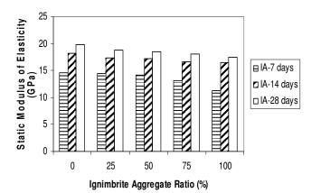
Figure 9. Effect of age, aggregate ratio on the static modulus of elasticity of IA concretes.
