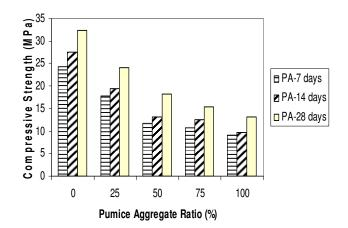
**Figure 2.** Effect of age, aggregate ratio on the compressive strength of PA concretes.
