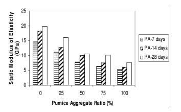
Figure 8. Effect of age, aggregate ratio on the static modulus of elasticity of PA concretes.
