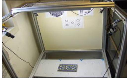
**Figure 5.** Setup system with orientation field and tile.
