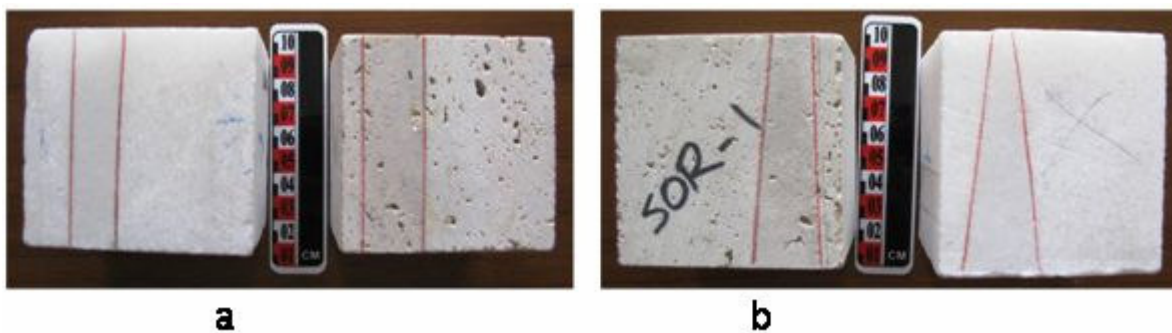
Figure 4. Appropriate and inappropriate abrasion surfaces in wide wheel abrasion tests. (a) Standard (appropriate) abrasion surfaces (b) Inappropriate abrasion surfaces.
